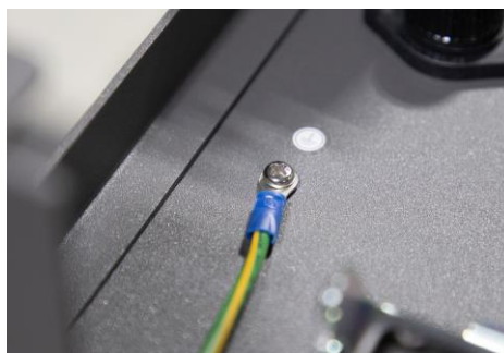
Figure 22: Grounding position for the control box
