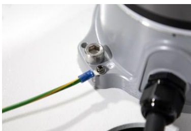
Figure 17: Grounding position for the robot
