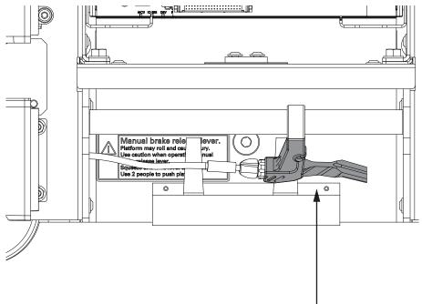
Ensure brake lever returns to original position after releasing.
