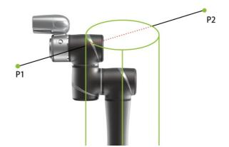
When the path crossing the Internal Singularity Point in Space, singularity will be triggered. Adjust the path and confirm it will not cross the Internal Singularity Point in Space.
