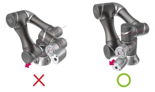
This example demonstrates how to avoid the rotational axes of the fourth and sixth joint being parallel, when the user need to move the robot according to tool Z-axis.
