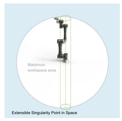
The maximum working range can be achieved when the third joint is almost at zero degrees
