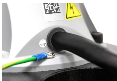
Figure 24: Securing the ground wire with the robot
