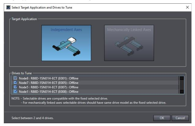
You can simultaneously perform Easy tuning on multiple compatible Drives, up to four Drives including the selected Drive.
