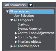
The parameters can be selected and displayed according to the categories predefined for each Drive series.
