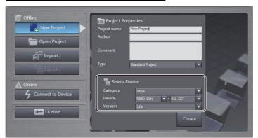
Note When the computer with Sysmac Studio running is directly connected to a Drive via USB, a new project can be automatically created for the connected Drive. To do so, click the **Connect to Device** button without opening a project in the above start page of Sysmac Studio. Refer to *Going Online from the Start Page of Sysmac Studio* on page 2-31 of 2-7 Online Connection Procedure on page 2-29 for details.
