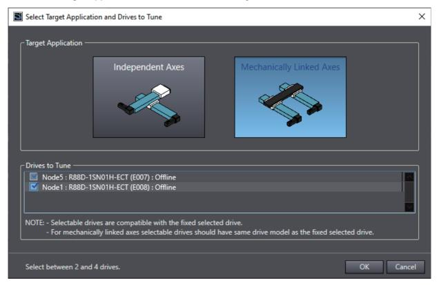
You can simultaneously perform easy tuning on multiple drives, up to four drives including selected drive. The compatible drives are the ones with the same model as the fixed selected drive.
