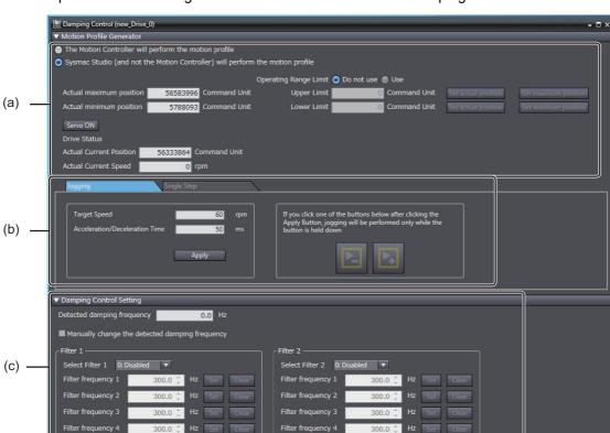
Set the operation command generator and conditions and also damping control conditions.
