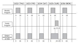
\*If a weekly program and a yearly program overlap in operation time, the output of the H5S is continuously produced without being interrupted.
