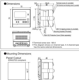
Note. The recommended panel thickness is 1 to 5 mm.
