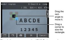
Check the area, press the [OK] Button, and then press the [TEACH] Button. The characteristic part and reference position for position compensation will be registered.
