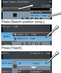
Place the object that is to be used as the measurement reference in front of the camera. Move the rectangle so that the characteristic part for position compensation is inside it.
