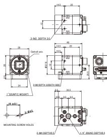
\* The base at the bottom of the camera can be mounted to the bottom, top, and both sides. Remove the base mounting screw (M2x7) and correct the mounting position. (Recommended mounting screw torque: 0.23 N·m)
