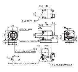
\* The base at the bottom of the camera can be mounted to the bottom, top, and both sides. Remove the base mounting screw (M2x7) and correct the mounting position. (Recommended mounting screw torque: 0.32 N·m)
