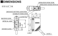
NOTE.1 VINYL INSULATED ROUND CORD 4dia 4CORES(CONDUCTOR CROSS SECTIONAL AREA 0.2mm2 INSULATION OUTSIDE DIAMETER: 11dia)
