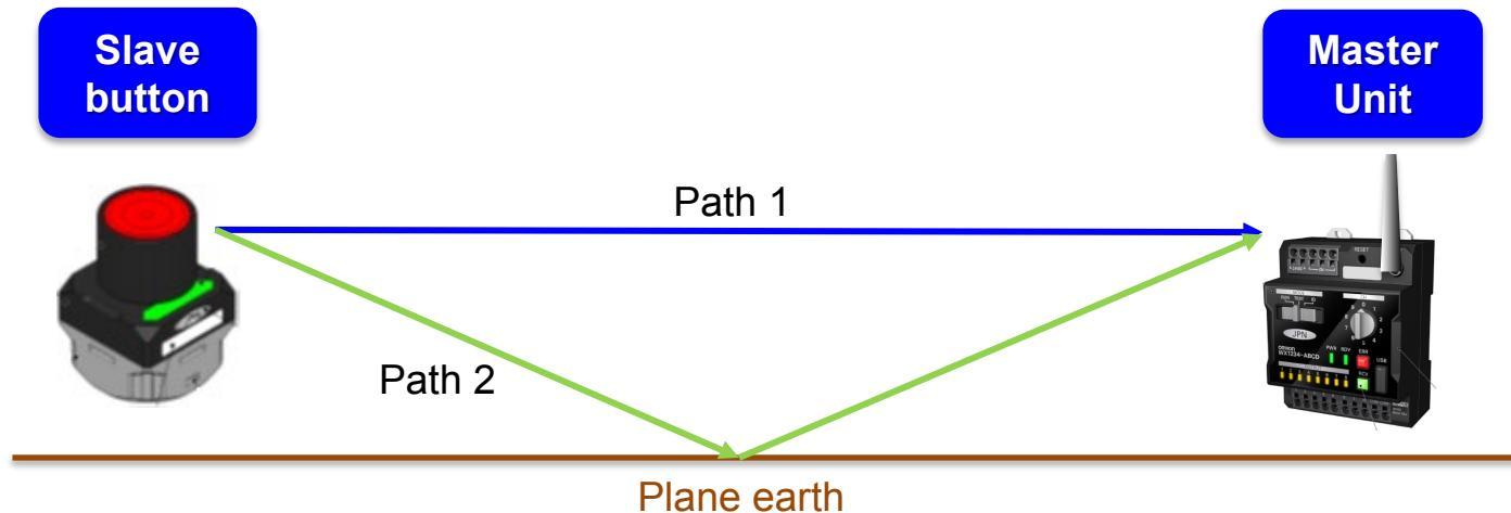
Phase shift (i.e., arrival time differences) occurs by the difference in path length. At the point where the phase shift is exactly opposite phase, the radio waves cancel each other and become a null point. At the position where it becomes a null point, the reception field strength is significantly lowered and it is difficult to receive.
