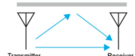
Direct wave and reflected wave strengthen or weaken each other.
