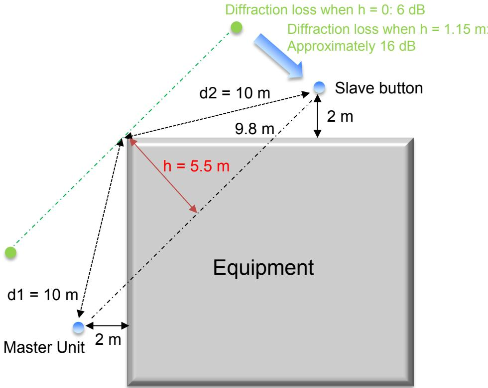
Example: knife-edge diffraction model
