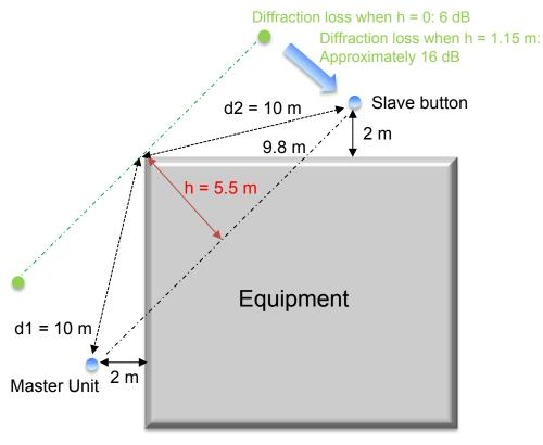
Example: knife-edge diffraction model
