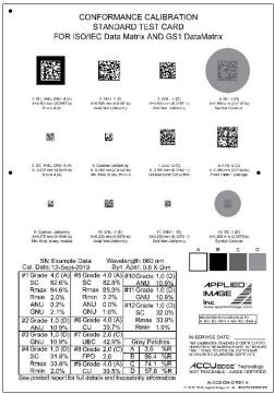
\*Note: If you have purchased an LVS-958X-DPM-HD Verification system (1.35" / 34.29 mm FOV), one of the above cards will be provided with the unit to use as a calibration card. Symbol 1 on the calibration card will be used to calibrate the system.
