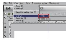
A check mark is placed on the left side of the menu display, and grids are displayed on the sheet.
