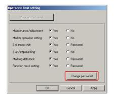
2 Enter the current password in [Current password] and the new password to be set in [New password] and [Confirm password], and click [OK].
