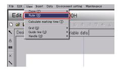
A check mark is placed on the left side of the menu display, and the rulers are displayed at the top and left sides of the sheet.
