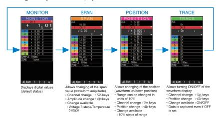
\* When ALL is set, setting values for CH1 is reflected on other channels. When CH1 is OFF, ALL Cannot be set.
