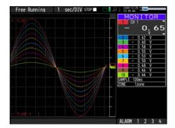
When in Free Running status, you primarily set up the system to capture data.
