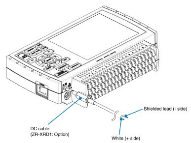
3 Connect the DC input side to the DC power supply.
