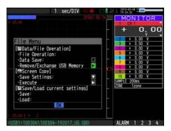
2 Move the cursor to Remove/Exchange USB Memory and press the ENTER key.
