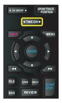
Press the left/right key of the TIME/DIV key to change the time axis display width.
