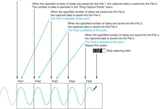
When capturing is stopped at the STOP point in the above, the File4 and the File 5 are remained. These files are consolidated into one file and it is saved. Then the ring capture is completed.
