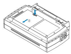
2 Attach the battery pack (ZR-XRB1).
