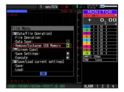
3 You can remove the USB memory device when the message is displayed.
