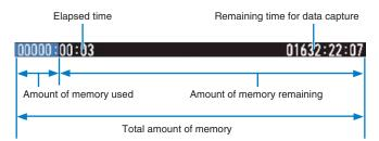
If, for example, 256 MB USB memory is inserted and about 96 MB is used before data capture, the total amount of memory is 256 MB, the amount of memory used is about 96 MB, and the amount of memory remaining is about 160 MB. As time elapses during data capture, the amount of used memory increases and the amount of remaining memory decreases.
