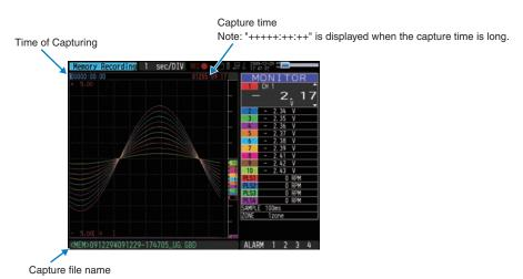
During data capture, data is captured into the Internal memory or USB device.
