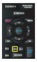
• This key is used to toggle between cursors A and B during replay.
