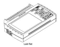
Do not block the air vent on the ZR-RX45, as this will cause malfunctioning.
