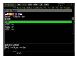
Use the  $\nabla\triangle$  key to move the cursor to the created "TEST" folder, and press the ENTER key.
