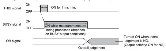
The timing for updating the OR signal and the ON time after judgement processing can be adjusted.
