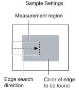
An edge is detected within the region according to set direction and color.
