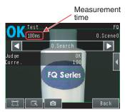
The measurement time is the time taken from when a trigger is input until when all measurement processes are executed.
