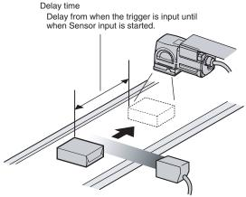
Trigger input Sensor
