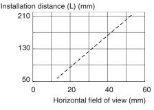
The optical chart indicates the horizontal field of view. The vertical field of view will be approximately 60% of the horizontal field of view.
