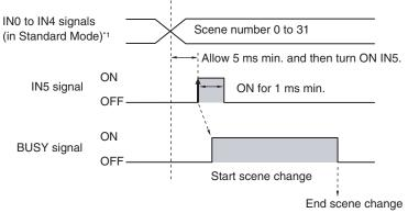
\*1: In Expanded Mode, specify scene numbers 0 to 15 using the IN0 to IN3 signals.
