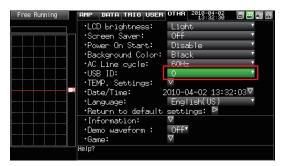
For ZR-RX45: Press the "MENU" key five times to open "I/F Settings". Input the "USB ID".
