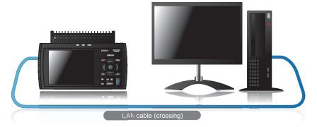
Use a straight cable to connect to a PC through a hub.
