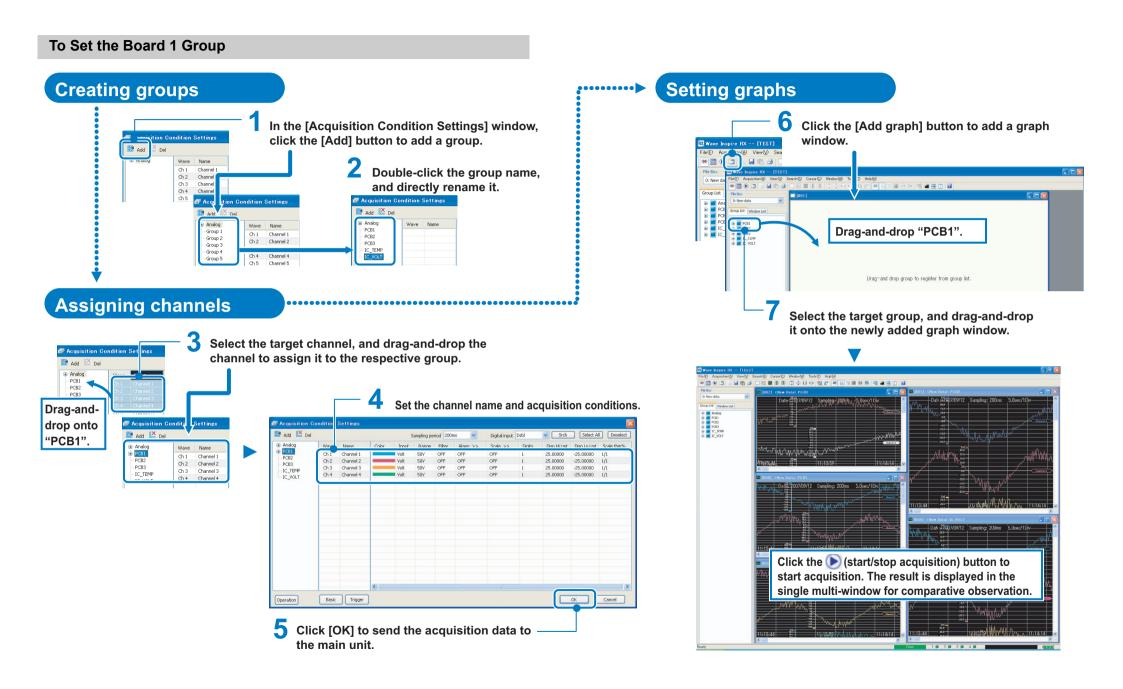
To Display the Measurement Data from Different Logger Types on the Same Graph
