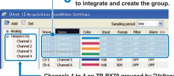
Channels 1 to 4 on ZR-RX70 grouped by "Voltage" and "Sampling Period (1ms)"
