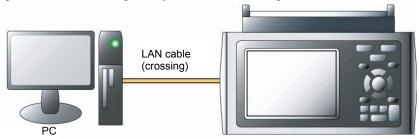
Use a straight cable to connect to a PC through a hub.
