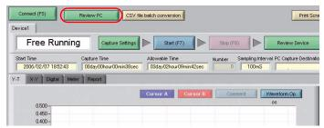
The file selection screen opens. Open the file to which the data was captured (p.48). A thumbnail waveform is displayed at the left of each file name, enabling you to confirm the data contents without opening each file.
