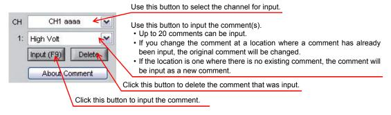
When On has been selected for Scroll: The comment is input at "Comment Input Pos" above the waveform graph.
