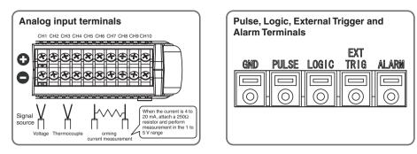
Refer to the channel numbers in the above figure to connect analog input terminals to the desired terminal.
