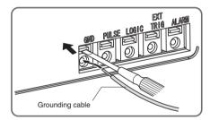
Use a flatblade screwdriver to push in the button above the ground terminal while connecting the grounding cable to the ZR-RX20. Connect the other end of the cable to ground.
