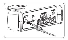
Connect the output side of the AC adapter to the AC adapter connector.
