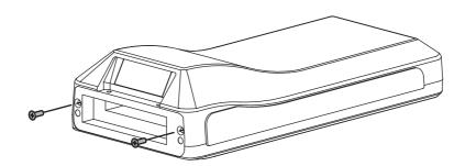
3. Secure the Protective Cover to the Handy Terminal with the four M2 screws provided with the Protective Cover.
