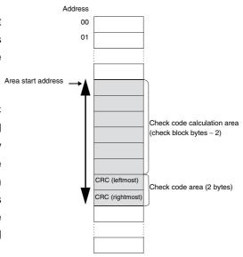
Calculate and write the check code using the Memory Check command (MD) after writing data and verify the check code before reading data. This enables detecting in advance data corruption in Tags that can occur while the Tags are not being accessed.
