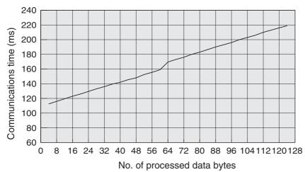
Read and write communications with Tags is performed in 4-byte units. This means that the communications time can be minimized by specifying the address and number of bytes so that the write start address is a multiple of 4.
