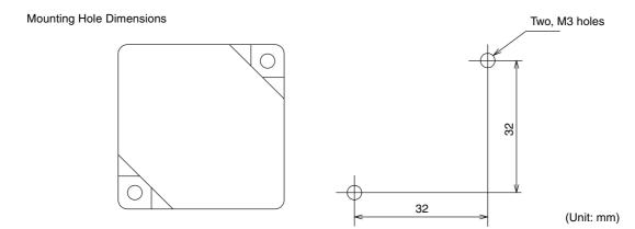
\* Tags must be mounted on flat surfaces. Do not mount Tags on curved surfaces.
