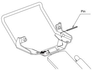
**4.** Secure the Protective Cover to the Handy Terminal with two #4-40 screws and two #2-56 screws.
