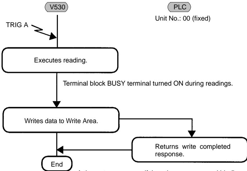
A timeout error occurs if there is no response within 5 s. An error message appears on the screen and the ERR (error) terminal turns ON.
