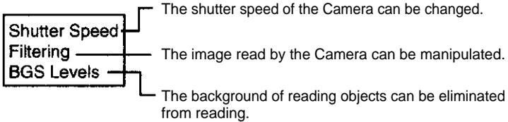
When adjusting the image on the monitor, change to a through image. The through images taken by the Camera are displayed so that the image can be adjusted while monitoring.
