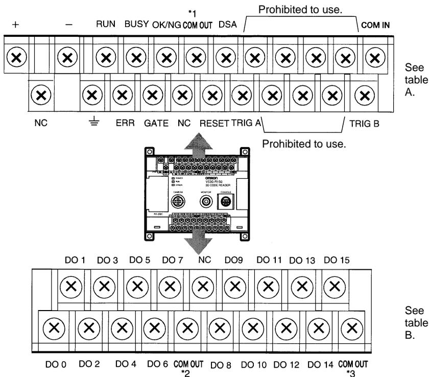
There are 3 kinds of COM OUT (\*1 to \*3) for each output terminal. Connect with reference to the following table.
