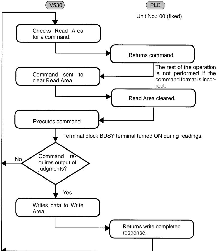
A timeout error occurs if there is no response within 5 s. An error message appears on the screen and the ERR (error) terminal turns ON.
