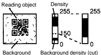
Image areas with densities of 149 or lower will not be read and the density will be changed to 0.
