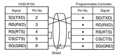
(\*) Pin numbers will depend on the CPU unit or Host Link Unit being connected. Refer to the manual for the Programmable Controller being connected.
