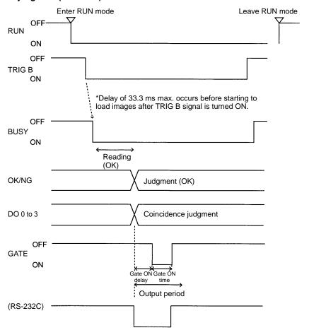
**Note** The output time to RS-232C changes according to the data volume and baud rate.
