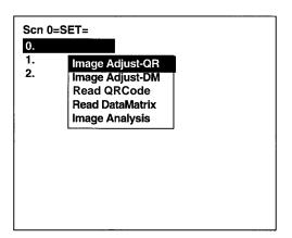
3 Move the cursor to the desired selection and press the ENT Key.
