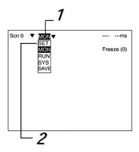
2 Move to SET using the Up Key and press the ENT Key.
