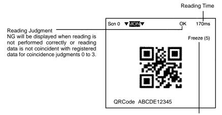
Displayed Images. Press the SHIFT + Up/Down Keys to switch images.
