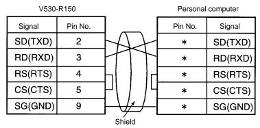
(\*) Pin numbers will depend on the type of personal computer connected. Refer to the manual of the personal computer.
