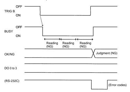
**Note** The output time to RS-232C will vary according to the data volume and baud rate.
