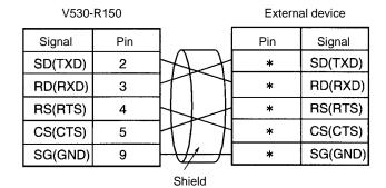
Note Pin numbers will depend on the external device being connected.
