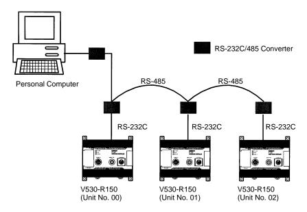
**Note** Refer to the manual of the converter for the number of V530-R150 that can be connected.
