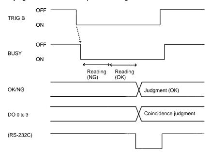
**Note** The output time to RS-232C will vary according to the data volume and baud rate.
