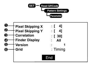
**1** Change the pixel skipping parameters used to search for a model. (1 to 20)
