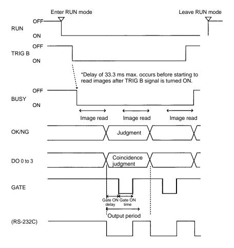
**Note** The output time to RS-232C changes according to the data volume and baud rate.
