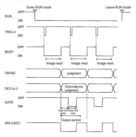
**Note** The output time to RS-232C changes depending on the data volume or baud rate.
