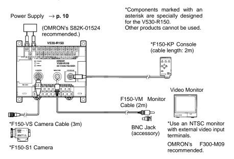
**Note** Turn OFF the power to the Controller before connecting or disconnecting cables. Connecting or disconnecting cables with power turned ON can damage peripheral devices.
