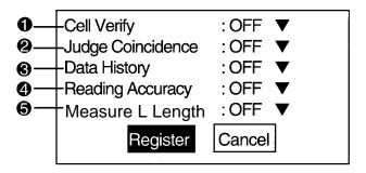
**Note** Cell Verify can be used together with Judge Coincidence, Data History, Reading Accuracy and Measure L Length, but no other combination can be used together.
