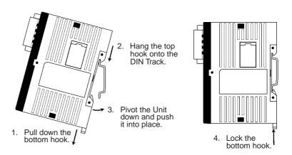
**Note** The DIN Track must be installed horizontally. If the Track is installed vertically, air will not flow properly through the Unit and the Unit may overheat.
