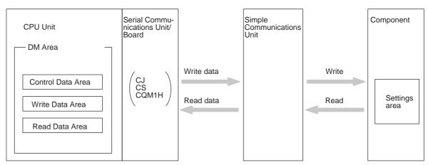
Interface between the Simple Communications Unit and PC
