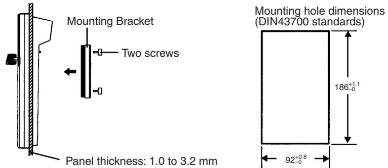
Allow at least 80 mm for the cable connector above the Programming Console.
