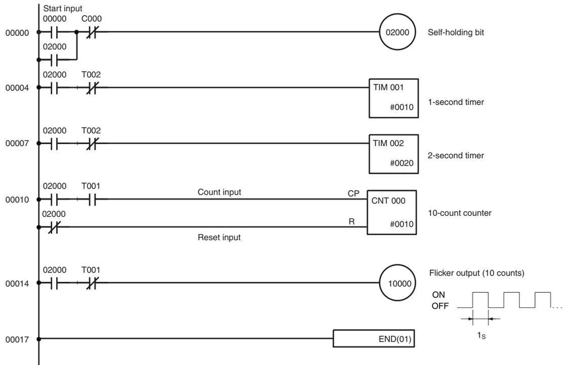
The mnemonic list for the example program is shown in the following table. The steps required to enter this program from a Programming Console are described in 7-4-4 Programming Procedures.
