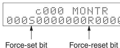
Note a) The status of displayed bits can be changed at this point. Refer to 7-3-20 *Binary Data Modification* for details.
