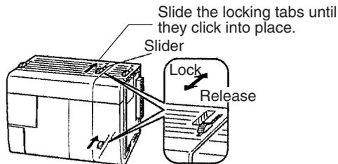
3. Attach the End Cover to the Unit on the far right side of the PC.
