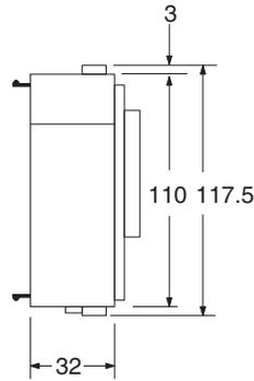
**Connector-type I/O Unit Side View**
