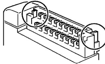
**Note** Confirm that the terminal block is securely locked before use.
