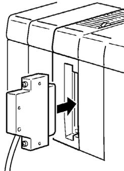
**Note** When using a cable connector with a locking mechanism, check that the lock is secure before use.
