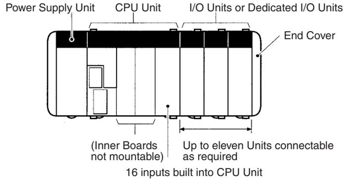
**CPU Block and Expansion I/O Block**
