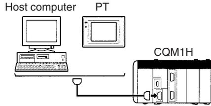
For details on cables required to connect the host computer to the CQM1H in Host Link Mode, refer to *3-6 Programming Devices*.
