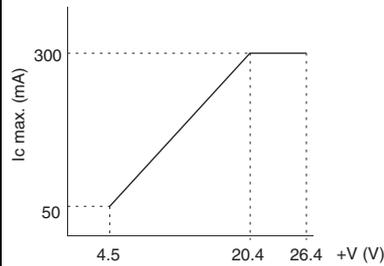
Max. Switch Capacity (Total for Unit)
