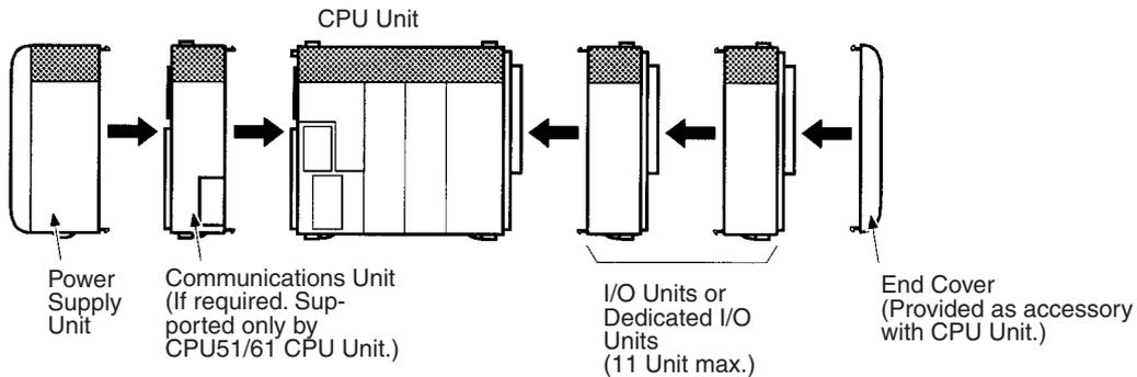
**CPU Block for Connection to Expansion I/O Block**
