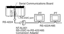
Connection to RS-422A/485 port of Serial Communications Board
