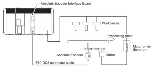
Detects angle of rotation and controls processing table.
