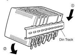
4. Lock the pins on the backs of the CQM1H Units.
