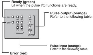
Lit when there is an error in the PC Setup settings for pulse I/O, or when operation is interrupted during pulse output.
