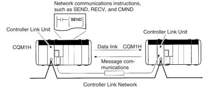
Baud rate: 2 Mbps; transmission distance: 1 km (when baud rate is 500 kbps); max. No. of nodes: 32. A maximum of 8,000 words per node can be sent for the CQM1H.
