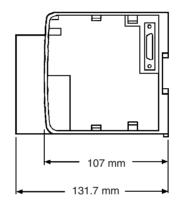
**Note** The depth of connector-type I/O Units is approx. 120 mm when pressure-welded connectors are used.
