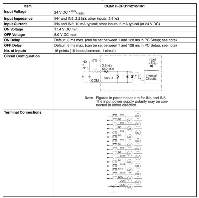
IR 00000 to IR 00015 are always allocated to the CPU Unit's 16 built-in input points.
