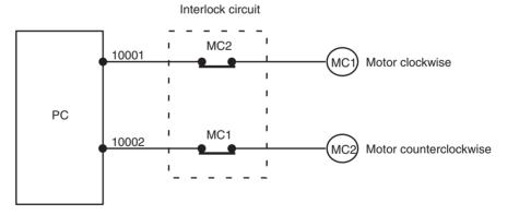
This circuit prevents outputs MC1 and MC2 from both being ON at the same time even if IR 10001 and IR 10002 are both ON, so the motor is protected even if the PC is programmed improperly or malfunctions.
