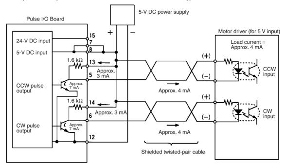
• The transistors of the internal circuits of the pulse output section are OFF when pulse output is stopped.
