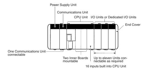
**CPU Block and Expansion I/O Block**
