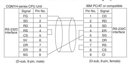
When preparing an RS-232C cable to be connected to the RS-232C port, use the following connector cables.
