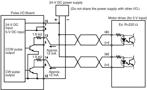
Note Here, a 5-V input motor driver is being used with a 24-V power supply. The internal resistance at the Pulse I/O Board (1.6 k $\Omega$ ) is thus used. Care must be taken to avoid problems caused by the drive current at the motor driver.
