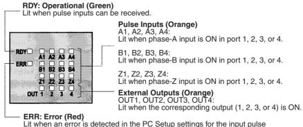
Lit when an error is detected in the PC Setup settings for the input pulse function, or when an overflow or underflow occurs in the high-speed counter's present value.
