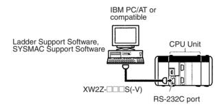
**Note** You can also connect to the RS-232C port on a Serial Communications Board.
