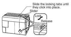
3. Attach the End Cover to the Unit on the far right side of the PC.
