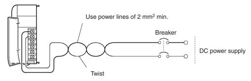
/!\ Caution Be sure that the DC power supply voltage remains within the allowed fluctuation range of 20 to 28 V DC.
