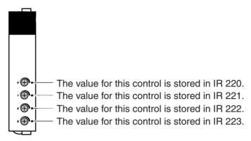
Caution While the power is turned ON, the contents of IR 220 to IR 223 are constantly refreshed with the values of the corresponding controls. Be sure that these words are not written to from the program or a Programming Device.
