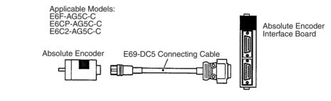
Applicable Cable: E69-DC5 Absolute Encoder Interface Board Connecting Cable (length: 5 m)
