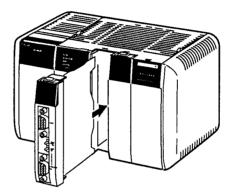
Caution Always turn the power OFF before installing or removing the Inner Board. Installing or removing the Inner Board with the power ON can cause the CPU Unit to malfunction, damage internal components, or cause communications errors.
