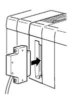
**Note** When using a cable connector with a locking mechanism, check that the lock is secure before use.
