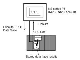
This section only explains how to open the PLC Data Trace Screen. Refer to 2-20 Special Functions in the NS Series Programming Manual for details on the specifications and operation of the data trace function.
