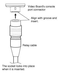
**Note** The Relay Cable (F150-VKP) is the cable used to connect the Video Board's console connector or to the console connector of an OMRON Vision Sensor.
