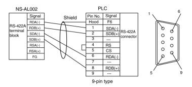
For details on processing shielded cable, refer to A-3-6 Handling the Shield on RS-422A/485 Cables.
