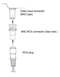
**Note** A BNC-RCA connector is provided with the Monitor Cable (F150-VM) for OMRON Vision Sensors. It is not provided with the Video Input Unit (NS-CA001).
