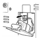
4. Connect the new battery connector, and insert the battery into the battery holder in the battery cover.
