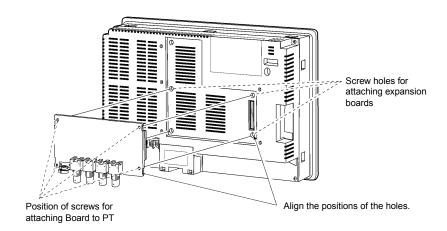
Push firmly on the connector end of the board to ensure that it is inserted sufficiently.
