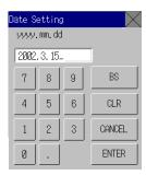
e) Press the time display area under the heading *Calendar Check*. A dialog box will be displayed. Input the time using a 24-hour clock in hours/minutes/seconds format.
