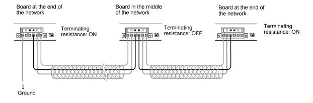
**Reference** • Terminals of the same type are connected internally. They can thus be connected to either the right or left half of the end Boards.
