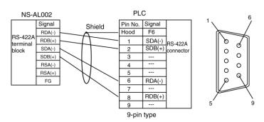
For details on processing shielded cable, refer to A-3-6 Handling the Shield on RS-422A/485 Cables.
