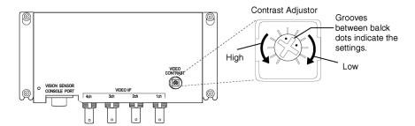
If turning the contrast adjustor too much, the image may be distorted. Turn the contrast adjustor in the opposite direction to remove the noise.
