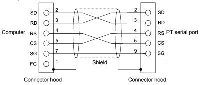
Use the following products to assemble the connecting cable.
