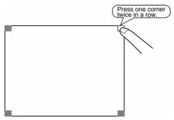
Make sure you press a corner where no functional object is displayed. If there is a functional object at the corner you press, the function of the functional object will be executed.
