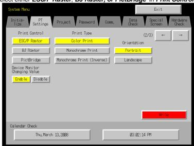
2. After setting, press the Write Button to save the setting.
