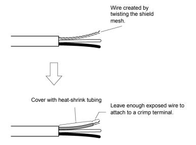
3. Strip the ends of the signal wires far enough to attach to the crimp terminals. Twist the wire strands together.
