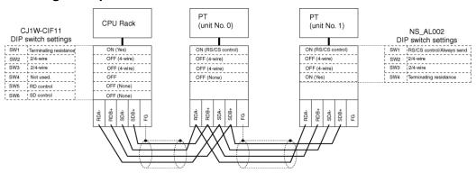
**Note:** Refer to A-3-6 Handling the Shield on RS-422A/485 Cables for information on processing the shield wire on the RS-442A/485 cable.
