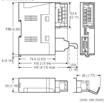
30 (W)  $\times$ 114 (H)  $\times$  100.2 (D) mm: with the RS-422A terminal block cover closed 30 (W)  $\times$ 114 (H)  $\times$  119.5 (D) mm: with the RS-422A terminal block cover open
