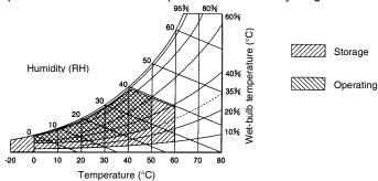
3. When a STN LCD display device is used, the display quality will decline (e.g., the contrast ratio will be reduced) if the temperature exceeds 40°C. Also, when the temperature drops, the response speed is lowered due to characteristics of liquid crystals.
