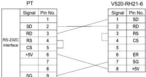
When connecting to the 5-V output of the PT's serial port, use a cable length of less than 2 m. If the cable is 2 m or longer, connect pins 7 and 8 of the Bar Code Reader to an external power supply.
