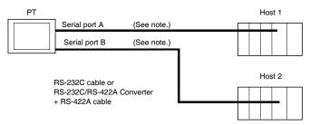
Note: Each port allows 1:N connection. NS-AL002 connects either serial A or serial B, but not both due to structural restrictions.
