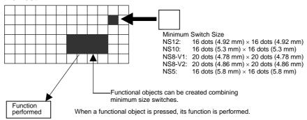
To ensure correct input operations, create touch switches so that they consist of at least two switches horizontally and vertically.
