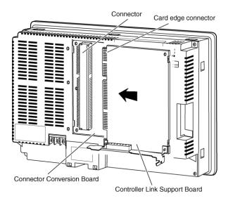
**Reference** Follow the steps given below if it is hard to insert the card edge connector to the connector on the connector conversion board.
