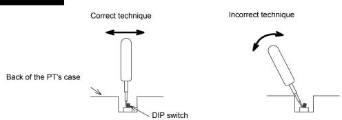
The DIP switch may bend or break if the tool is incorrectly levered against the PT's case as shown in the diagram.
