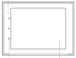
The brightness of the indicator will change according to the brightness setting of the backlight. The brightness will not change on PTs with lot number 30114 or earlier.
