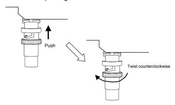
2. After unlocking the BNC socket, pull it out.
