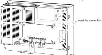
Align the cover's screw holes with the screws and mount the cover.
