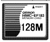
**Note** Use a Memory Card recommended by OMRON. Incorrect operation may occur if a non-recommended memory card is used.
