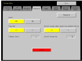
3. After making the required settings, press the **Write** Button to save the settings.
