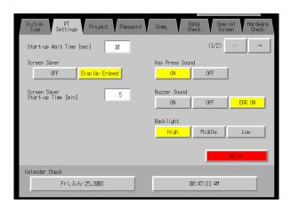
d) Press the date display area under the heading *Calendar Check*. A dialog box will be displayed. Input the date in yyyy/mm/dd format.
