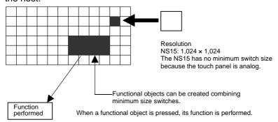
To ensure correct input operations, create touch switches so that they consist of at least 32 x 32 dots.
