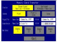
6. Specify the direction of the transfer (download or upload), the transfer contents (project, project and system program, or system program), and bank. The IPP file name and system version that are stored in both the specified bank of the Memory Card and the PT will be displayed in the Project File and System Version fields. After confirming the details, press the Go Button.
