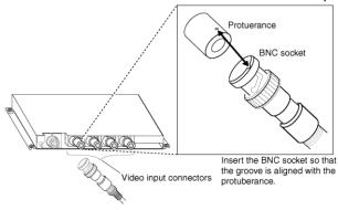
2. After inserting the BNC socket, twist it clockwise until it locks into place.
