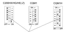
RS-232C Communications Conditions Setting Set pin 5 of the DIP switch to OFF to enable the PLC Setup Area settings.
