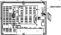
Tighten the Memory Card bracket screw. The tightening torque is 0.6 N⋅m.
