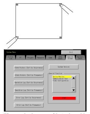
When pressing the corners of the touch panel, however, first press a corner that does not have a functional object displayed. If the position of a functional object is pressed, its function will be performed. If the command button for switching screens is kept pressed after the screen has been switched, it will be detected as if the button has been released.
