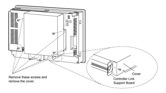
2. Disconnect the Controller Link Support Board from the connector conversion board. Hold both ends of the Controller Link Support Board and pull out straight.
