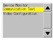
2. Press the Communication Test Button to switch to the Communications Test Screen.
