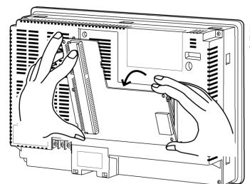
Hold the four corners of the Board and detach upper side first.
