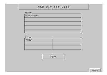
A list of USB devices currently connected and a list of USB devices supported by the NS Series are displayed. Press the **Update** Button to reconfirm the connected USB devices and refresh the display.
