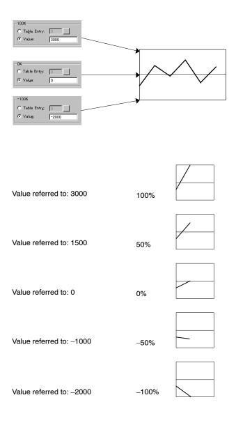
If the 100% value, 0% value, and -100% value are set using numeral memory table entries as indicated below, the percentage value of the reference value is calculated according to the value stored at the specified address.
