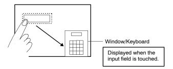
• It is possible to create a temporary input field at the same time as numeric keys are arranged in the window/keyboard.
