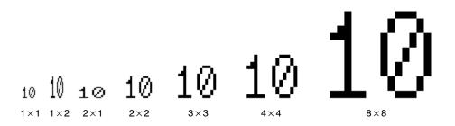
Reference: With the NT21 and with the NT31, NT31C, NT631, and NT631C "-V1" and above, numbers of 2×2 or larger scale are automatically displayed in 32 dot font.
