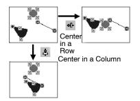
However, if a touch switch (including elements, such as thumbwheels, alarm lists/histories, that contain touch switches within themselves) is included in the selected elements, the touch switch will take precedence for alignment and the other elements will be aligned to the touch switch as follows:
