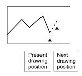
Pen Reco: The latest drawing position is fixed and the entire graph moves in the direction set for [Direction].
