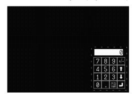
**Reference:** With NT30, 30C, NT620S, NT620C, and NT625C, screen numbers of the screen where a window/keyboard screen can be created are restricted to 1900 to 1979. With the NT21, NT31, NT31C, NT631, and NT631C, however, a window/keyboard screen can be created for any screen number as with a standard screen (1 to 3999).
