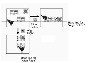
**Reference:** • Alignment function can be used also in the Edit Object mode. By using this function in this mode, position of the lamp/touch switch label or image/library
