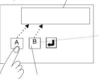
The input field and the control code input touch switch are automatically correlated. Insertion of a character string is automatically processed.
