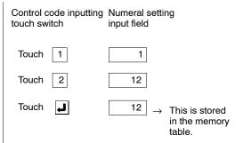
• The procedure for creating a control code input touch switch is shown below.
