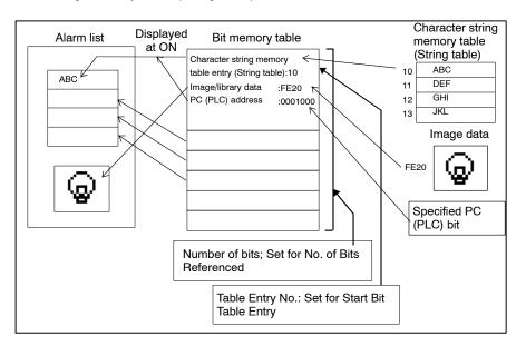
An alarm list element is used in combination with bit memory table entries. How they function is shown below:
