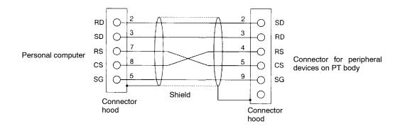
Note Connect the shield wire to the connector hood at both the personal computer and at the PT.
