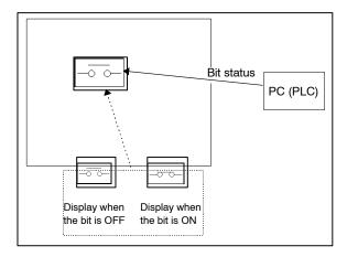
(1) The image data or the library data is switched to be displayed according to the status of the allocated PC (PLC) bit.
