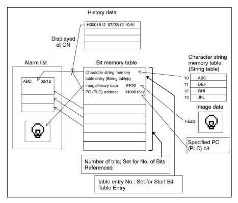
• An alarm history element is used in combination with the bit memory table entry. How they function is shown below:
