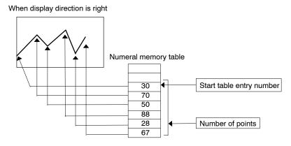
• The intervals between numeral memory table entries in a broken-line graph can be set as even or uneven, as desired, with the [Interval Type] line property.
