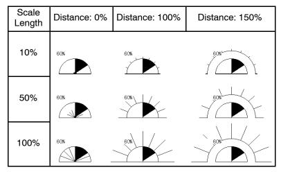
Scale is always displayed at the front of meter. Therefore, when type is set to a Needle, the needle may be invisible if meter and scale are overlapped.
