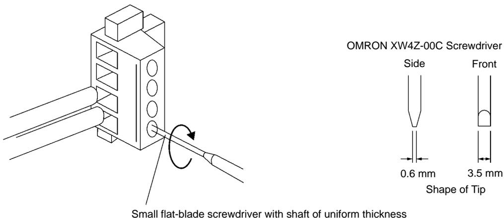
3. With the cable attached, connect the connector to the Controller. Align the cable connector with the connector at the Controller, and firmly push it all the way in. Then tighten the screws to a torque of 0.3 N•m.
