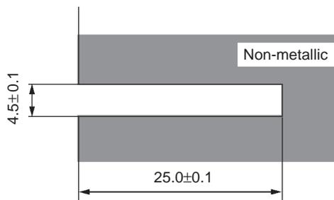
**Note** The diameter of the ID Tag itself is 4 mm. If the ID Tag is mounted using adhesive, the adhesive must fit into the space between the ID Tag and the panel, so the hole diameter should be approximately 4.5 mm.
