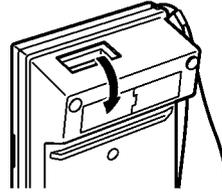
2. Connect the square connector to the Programming Console. Press in the square connector securely until the lock lever clicks.
