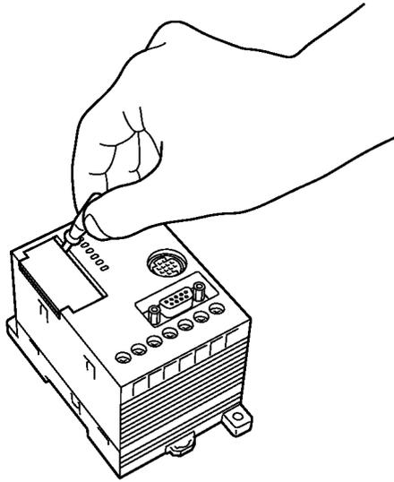
Under the cover, there are two node number switches (SW1 and SW2), two DIP switches (SW3 and SW4), and a port to connect the Programming Console.
