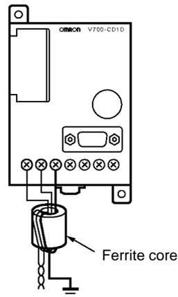
4. If the synchronous cable is used, wind only the power supply wires around the ferrite core as shown below.
