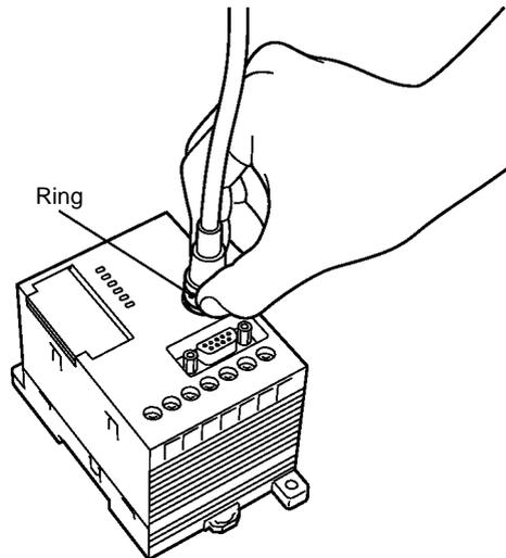
Hold and pull the ring straight upwards.
