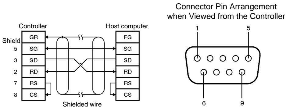
The diagram on the left-hand side indicates that the shielded wire is grounded on the Controller side.
