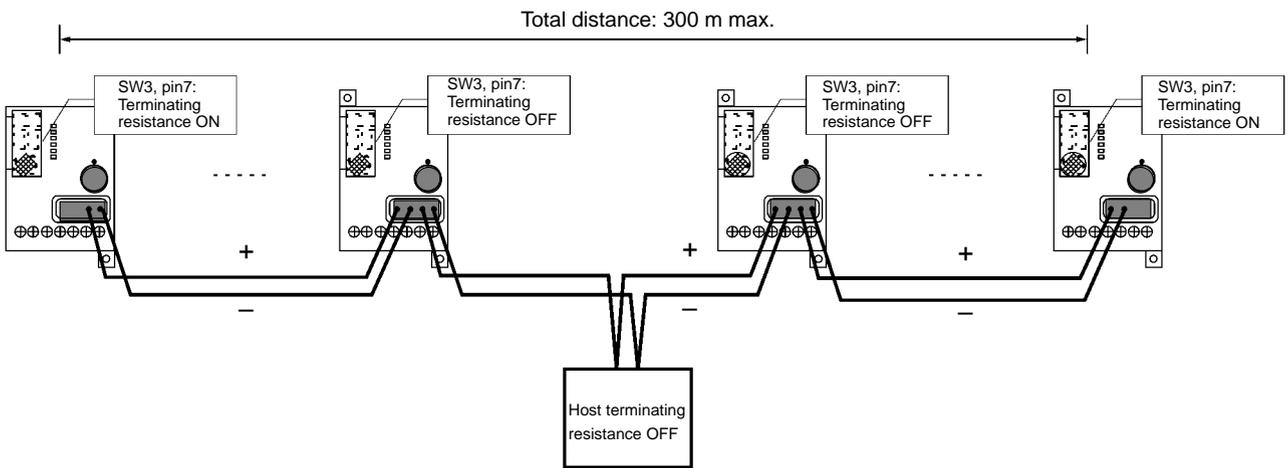
**Note** If the recommended cable is not used, wire a synchronous cable in parallel with the RS-485 interface cable. Even if this done, noise immunity will be reduced if the cable is wired as shown in example 2 or 3 below.
