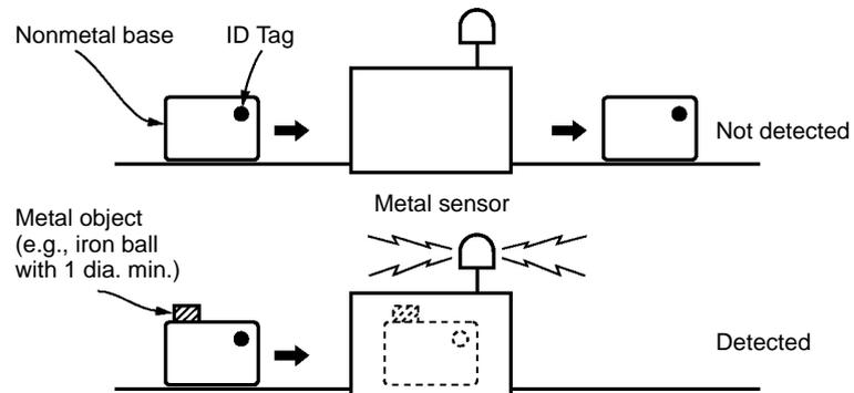
The ID Tag will not be detected by the metal sensor if its sensitivity is set to a normal level (i.e., the sensitivity is set for the detection of iron balls each of which is 1 mm or more in diameter). The ID Tag will not have a negative influence on the functions of the metal sensor, either.
