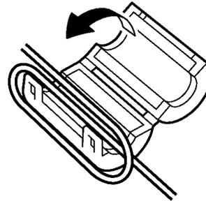
3. Close and press the ferrite core until the ferrite core clicks so that the ferrite core will be locked.
