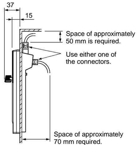
Consider the space required for the cable when mounting the Programming Console to the panel.
