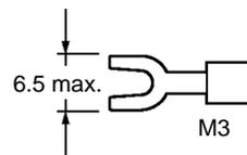
Tighten each screw to a torque of approximately 6 kgf • cm.
