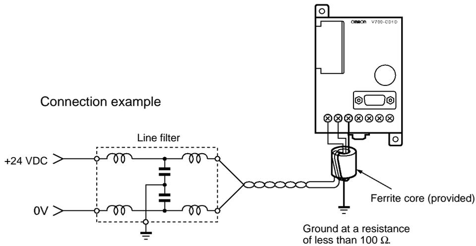
The power supply and ground terminals use M3 set screws. The following type of solderless terminals can be connected to these terminals. Tighten each screw to a torque of approximately 6 kgf • cm.
