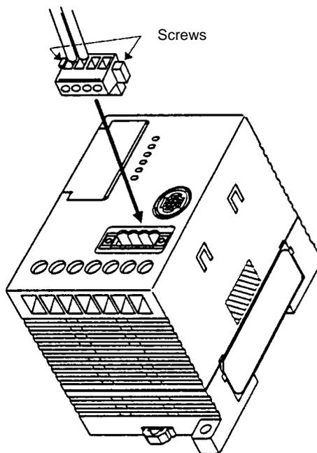
4. To remove the connector, first completely loosen the two screws and then grasp the protruding parts of the connector and pull it straight out. If it is difficult to pull out, then press down on the Controller while pulling on the connector.
