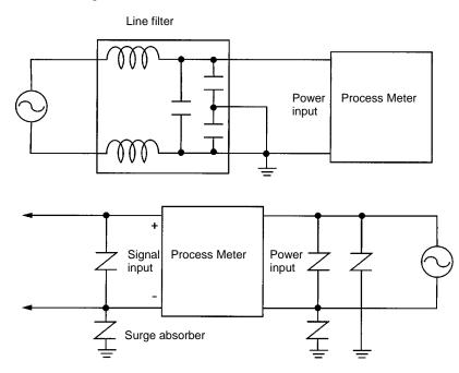
• Countermeasures for protecting the product against inductive noise produced from the input line.
