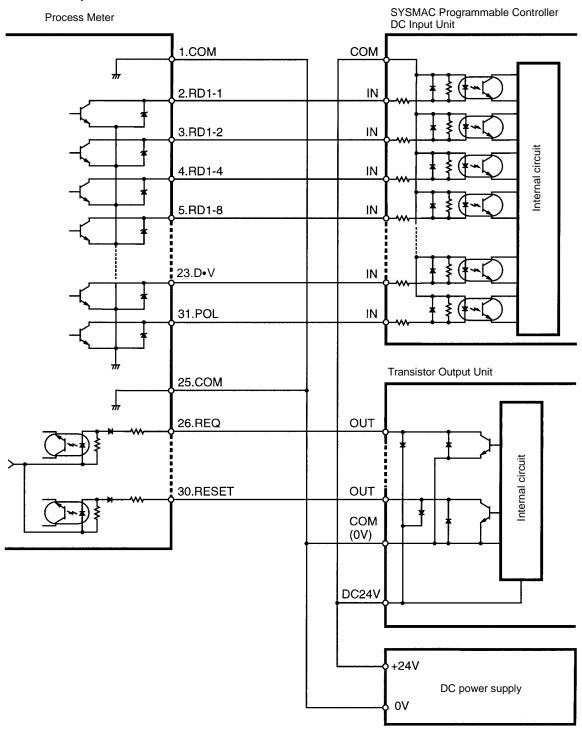
Note 1. Connect RD2-1 through RD2-4, RS3-1 through RS3-4, RD4-1 through RD4-4, and RD5-1 through RD5-4 in the same way as RD1-1 through RD1-4.
