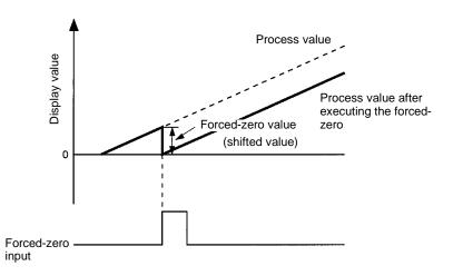
• The following is the relationship between the process value after scaling and display value after the process value is shifted to zero.
