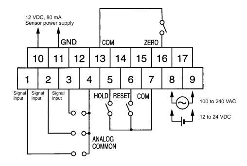
Note Terminals 7 to 13 are connected internally.
