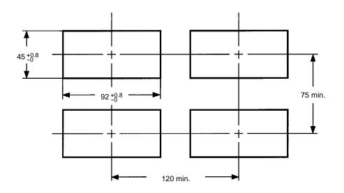
Recommended panel thickness is 1 to 3.2 mm.
