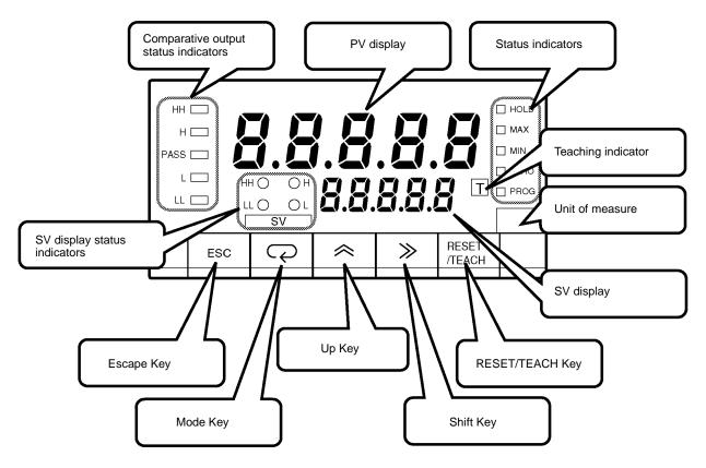
Five-digit (-19999 to 99999), seven-segment, 14.2-mm-high LED display with a programmable decimal point.
