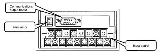
K3NX with RS232C + Transistor Output Board, K31-FLK4 K3NX with RS-422 + Transistor Output Board, K31-FLK6
