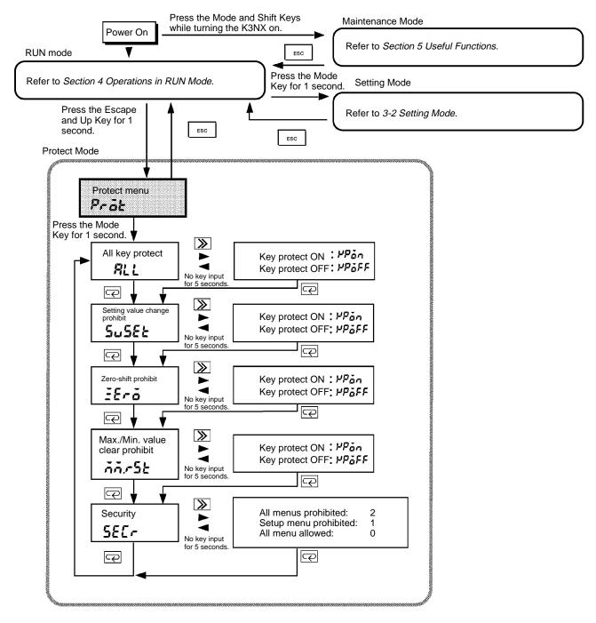
**Note** 1. The K3NX stops measurement in setting mode.
