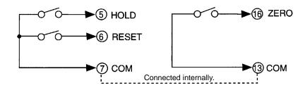
Connect hold signal (HOLD) input to terminal 5.
