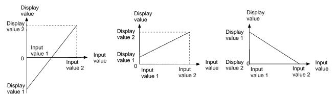
For example, if a sensor with 4- to 20-mA output is connected to the K3NX and the K3NX is set so that it will display "0" for 4-mA input and "999" for 20-mA input, the following will be the relationship between input and display values.
