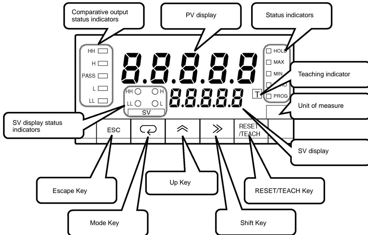
Five-digit (-19999 to 99999), seven-segment, 14.2-mm-high LED display with a programmable decimal point.
