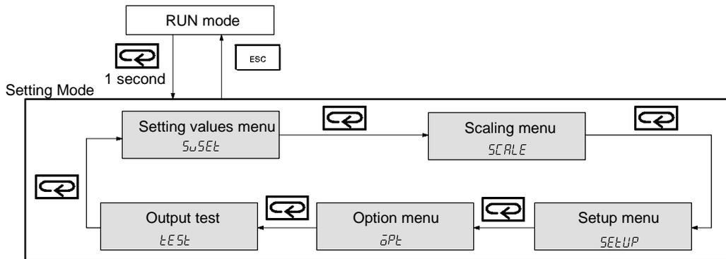
3. Press the Mode Key for more than one second to display 0, which is a simulated input value.
