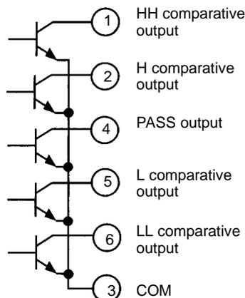
The following transistor output conditions are required.
