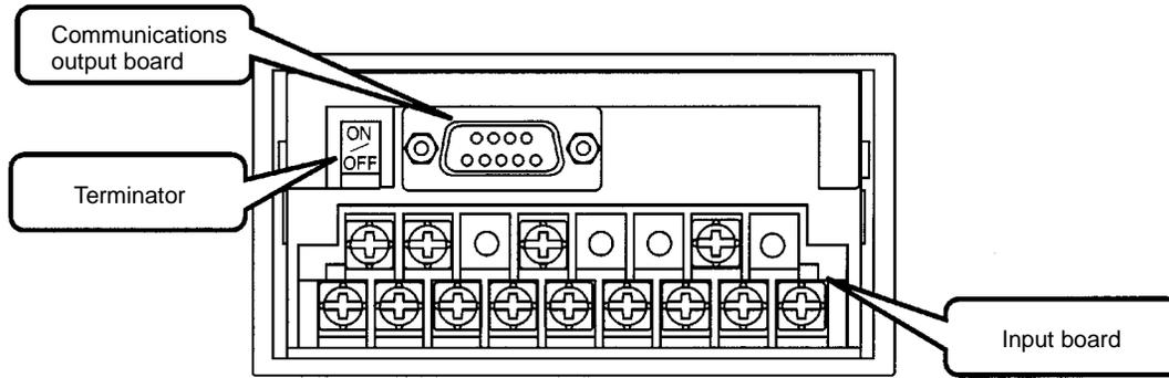
**K3NX with RS232C + Transistor Output Board, K31-FLK4**
