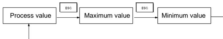
Used to return from the setting, protect, or maintenance mode to the RUN mode. This key is also used to return to the previous operation during the setting, protect, or maintenance mode.
