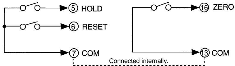
Connect hold signal (HOLD) input to terminal 5.
