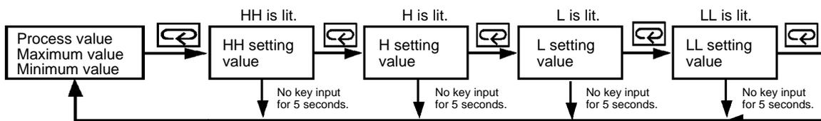
In the RUN mode, this button terminates the measurement process and allows you to enter the setting mode, advancing through the menus and parameters.
