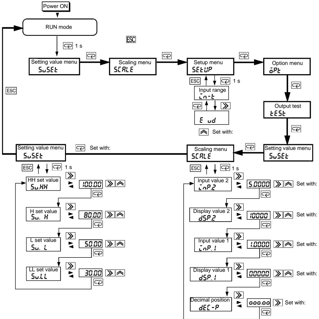
With the K3NX-AA□C-L4, the input of 0 to 10 A can be converted and displayed within a range of 0.000 to 10.000 and can be output in the range of 4 to 20 mA in proportion to the change in display value according to the following conditions.
