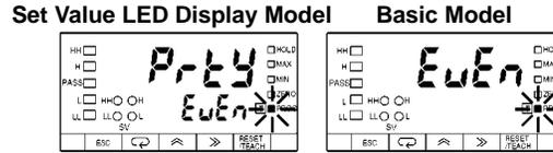
10. Press the Up Key to display  $n\bar{o}nE$ . The setting will be validated automatically if no change is made for five seconds. The  $Prty$  parity bit setting will be displayed again.
