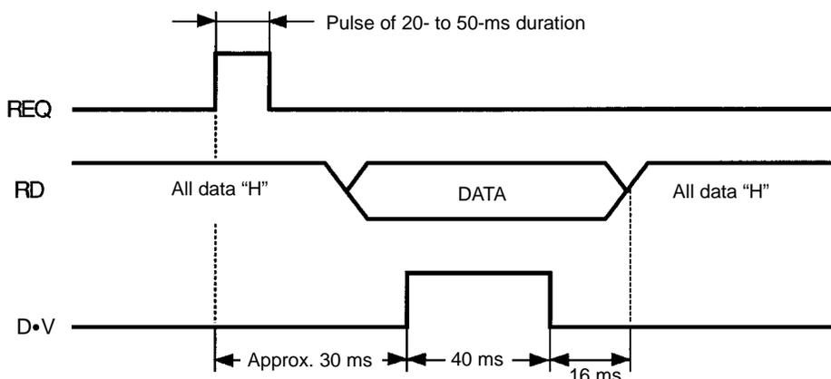
The REQ signal must be kept ON as shown below if the K3NX has continuous data output.
