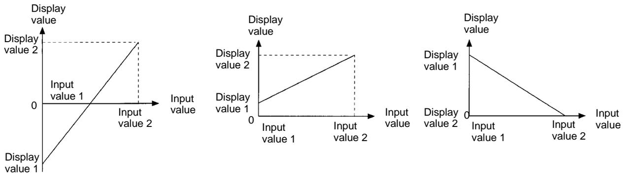
For example, if a sensor with 4- to 20-mA output is connected to the K3NX and the K3NX is set so that it will display "0" for 4-mA input and "999" for 20-mA input, the following will be the relationship between input and display values.
