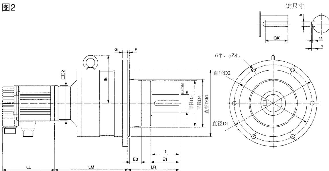
● 带标准齿轮的3,000-r/min扁平型伺服电机 (100 W~1.5 kW)
