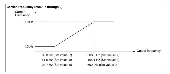
• The Inverter cannot maintain rated output current with the carrier frequency set to a value higher than the default one.
