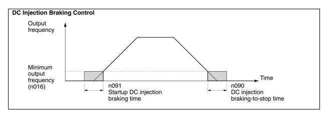
**Note** It is normally not necessary to change the settings of n173 (Proportional Gain for DC Control) and n174 (Integral Time Constant for DC Control). Adjust n89 to n91 to achieve optimum performance.
