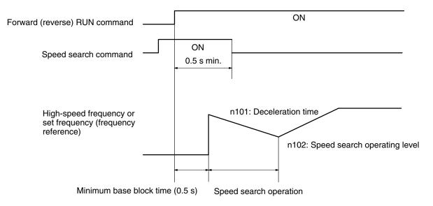
**Note** For 5.5- and 7.5-kW Inverters only, the speed search function can be adjusted by setting parameters n101 (speed search deceleration time) and n102 (speed search operating level). If the speed search cannot be executed properly using the default setting, lengthen the deceleration time or lower the operating level. To reduce the speed search time, check with the application while either shortening the deceleration time or raising the operating level.
