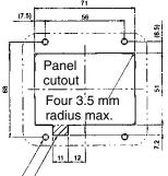
Cut off the area marked by diagonal lines to make room for the CN2 connector.
