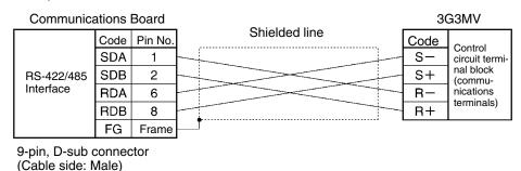
**Note** Turn the terminal resistance of all the Inverters to ON for RS-422 communications. Refer to page 2-18, *Selecting RS-422/485 Termination Resistance* for details.
