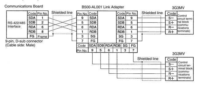
**Note** Be sure to set the terminal resistance of only the Inverter at each end to ON and that any other Inverter to OFF. Refer to page 2-18, *Selecting RS-422/485 Termination Resistance* for details.
