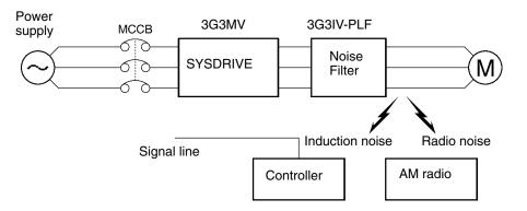
Induction Noise: Electromagnetic induction generates noise on the signal line, causing the controller to malfunction.
