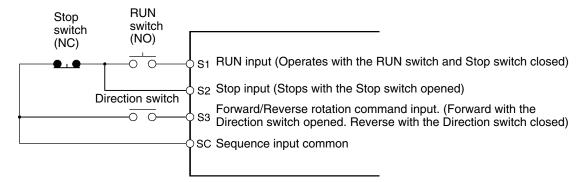
Note Set parameter 052 to forward/reverse rotation command 0 for 3-wire sequence input.
