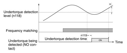
**Note** Undertorque detection will be canceled if the value increases from the detection level by approximately 5% of the Inverter rated current (or motor's rated torque).
