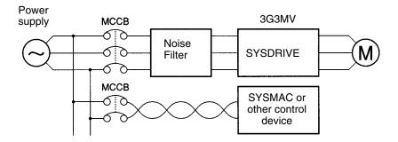
**Note** Use a noise filter designed for Inverters. A general-purpose noise filter will be less effective and may not reduce noise.
