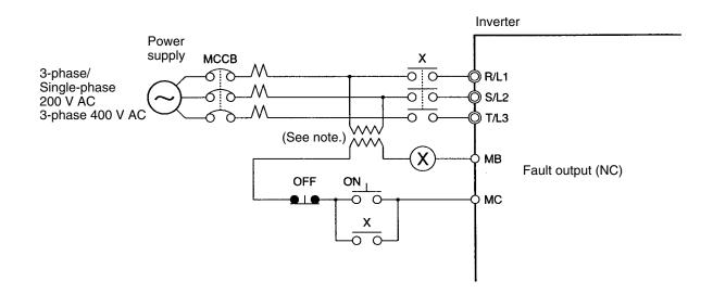
Note Use a 400/200 V transformer for a 400-V model.
