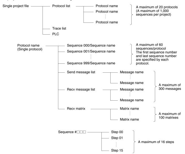
**Note** The standard system protocol incorporated by the Communications Board cannot be edited or transferred. To make use of the standard system protocol, copy it to the project file and edit it. In *7-9-4 Creating a Project File*, an example to create a new project file is shown without making use of the standard system protocol.
