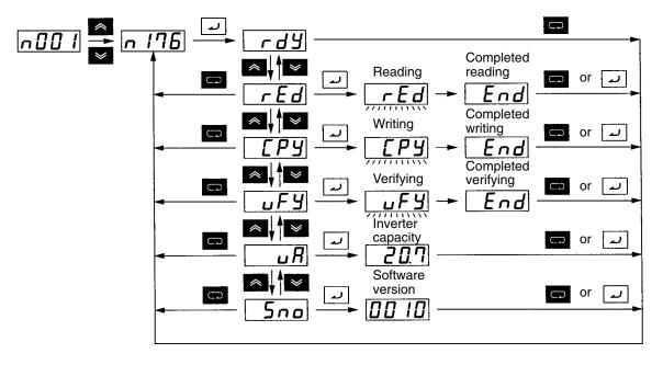
**Note** The following display is an example of the capacity displayed. The values in parentheses indicate the capacities for European motors.
