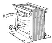
The DC Reactor suppresses harmonic current generated from the Inverter and improves the power factor of the Inverter. The DC Reactor suppresses harmonic current more effectively than the AC Reactor. Furthermore, the DC Reactor can be used in combination with the AC Reactor.
