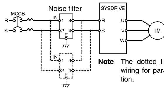
**Note** The dotted lines indicate wiring for parallel connection.
