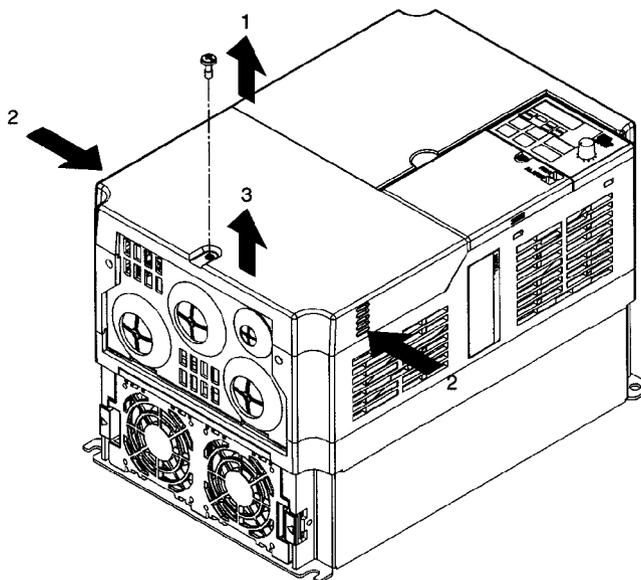
**Note** None of the following 200-V models have a terminal cover. Instead, the front cover is used as a terminal cover.
