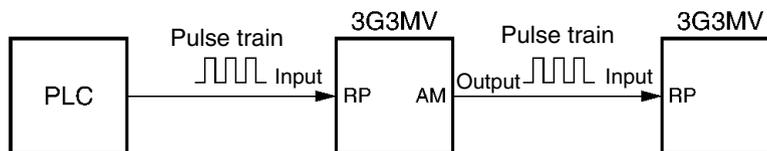
● Frequency Reference Input by PLC Pulse Train
