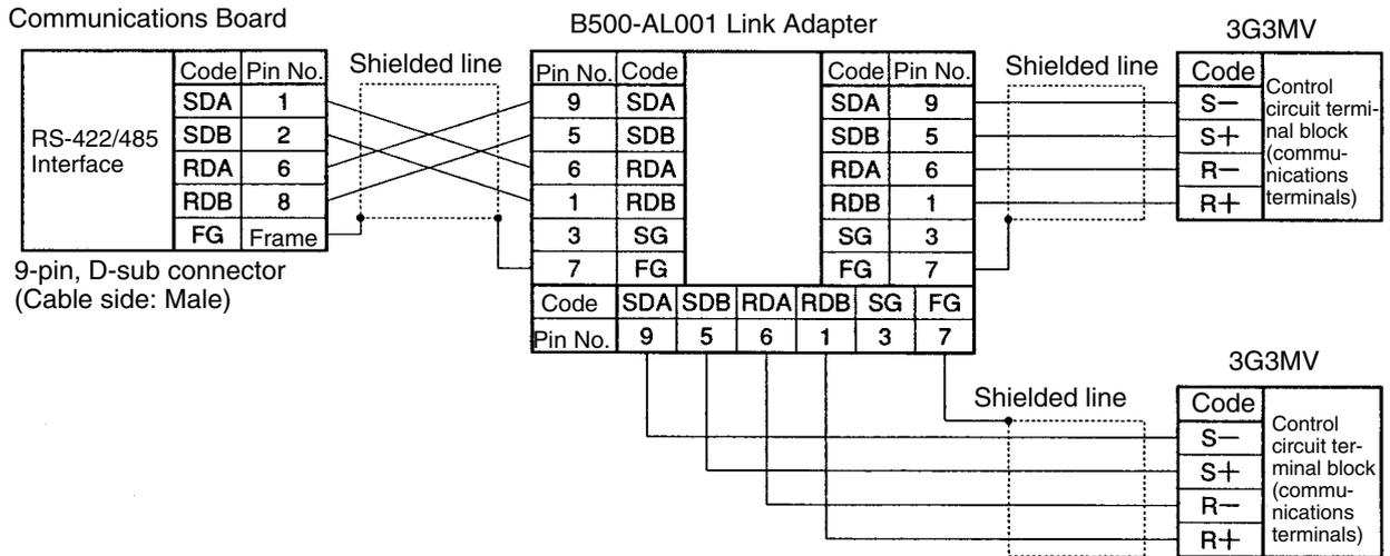
**Note** Be sure to set the terminal resistance of only the Inverter at each end to ON and that any other Inverter to OFF. Refer to page 2-18, *Selecting RS-422/485 Termination Resistance* for details.
