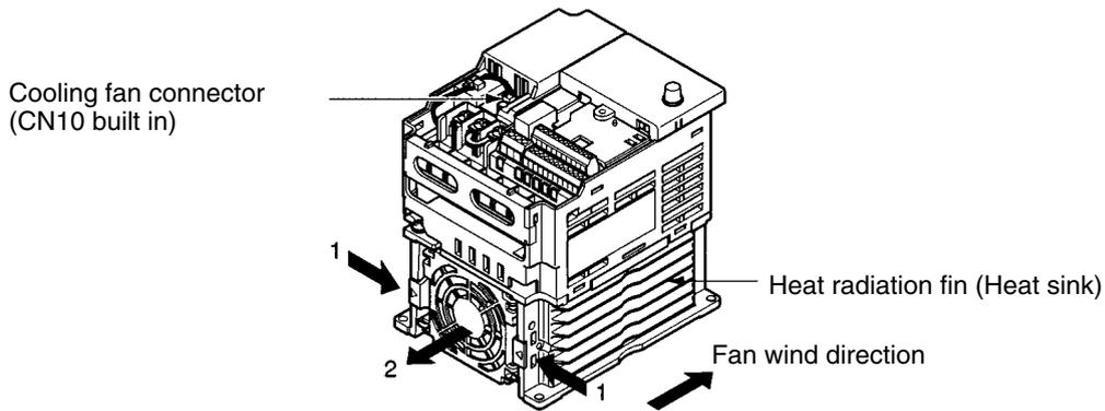
2. Press the left and right sides of the fan cover located on the lower part of the radiation fin in the arrow 1 directions. Then lift the bottom of the Fan in the arrow 2 direction to remove the fan as shown in the following illustration.
