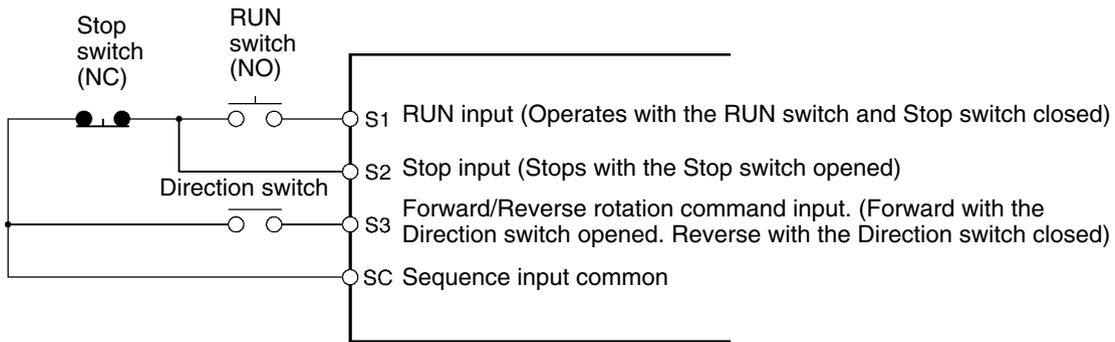
**Note** Set parameter 052 to forward/reverse rotation command 0 for 3-wire sequence input.
