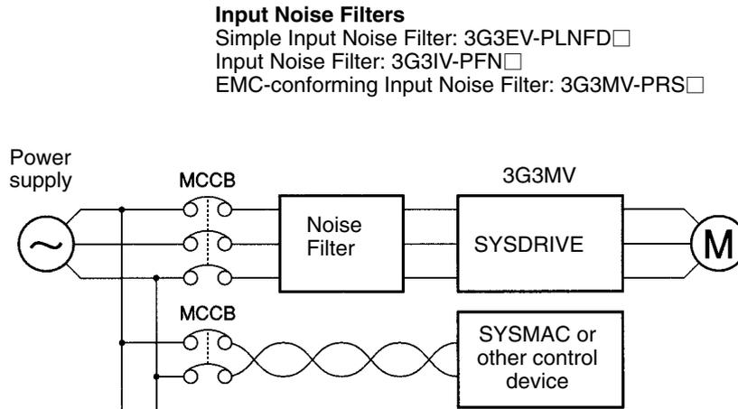
**Note** Use a noise filter designed for Inverters. A general-purpose noise filter will be less effective and may not reduce noise.
