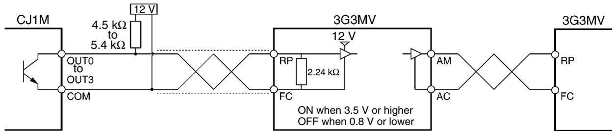
**Note** Use twisted pair shielded wire no longer than 5 m for pulse train input lines in order to suppress noise.
