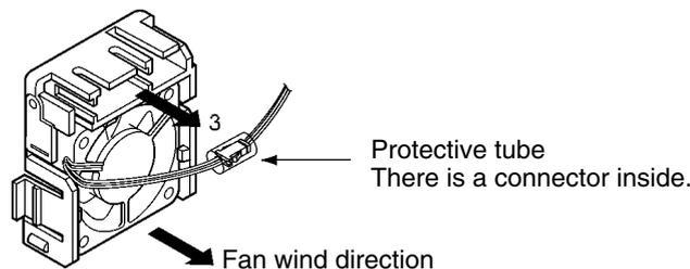
3. Slide the protective tube and remove the internal connector.
