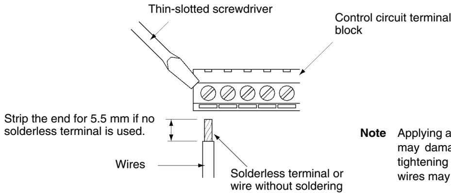
**Note** Applying a torque of greater than 0.5 N•m may damage the terminal block. If the tightening torque is insufficient, however, wires may be disconnected.
