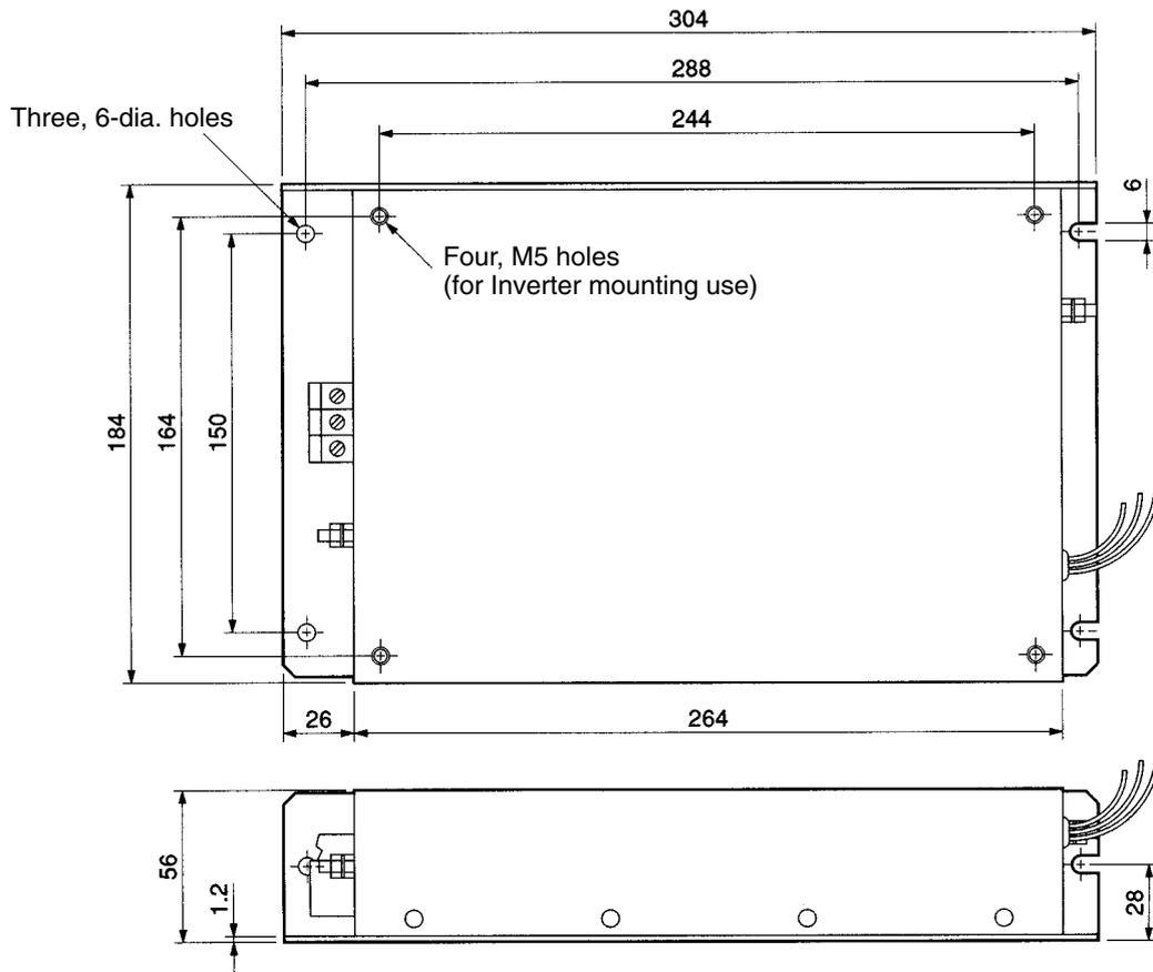
Noise Filters for Single-phase 200-V AC Models
