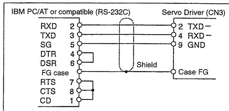
Make sure that the cable length is no longer than 2 m.
