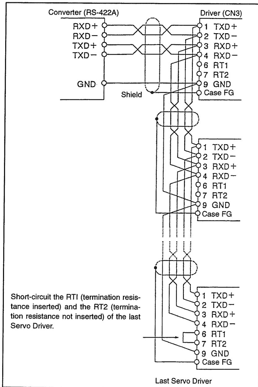
When connecting to the RS-422A converter ports for the purpose of extending the cable length, etc., wire according to the diagram above. Make sure that the cable length is no longer than 30 m.
