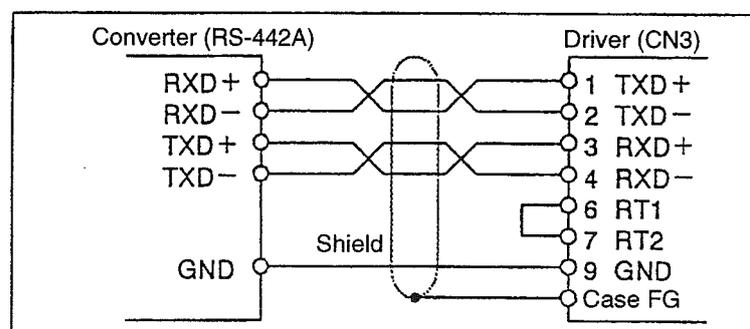
When connecting to the RS-442A converter ports for the purpose of extending the cable length, etc., wire according to the diagram above. Make sure that the cable length is no longer than 30 m.
