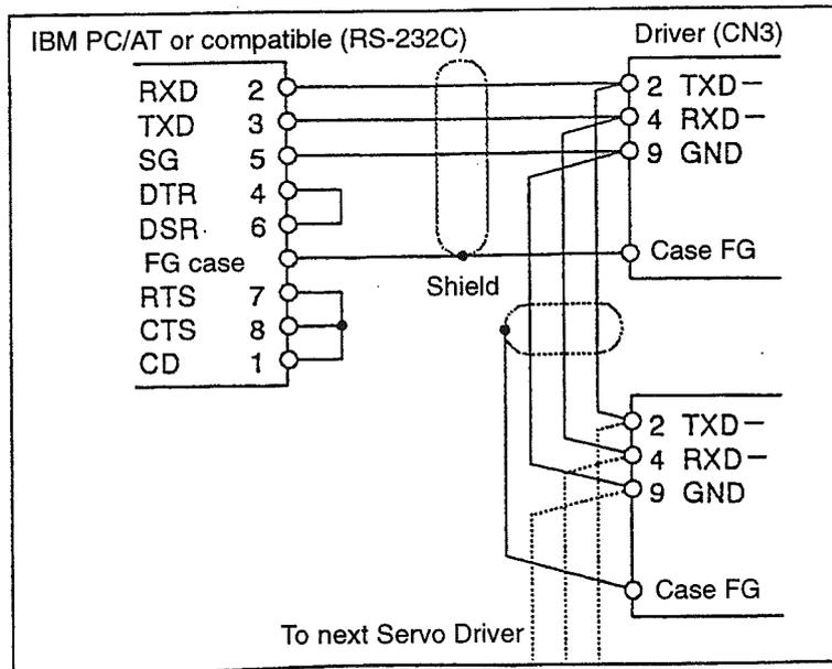
Make sure that the cable length is no longer than 2 m.
