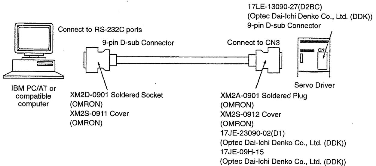
● Connecting to One Servo Driver (Connecting Directly to RS-232C Ports)
