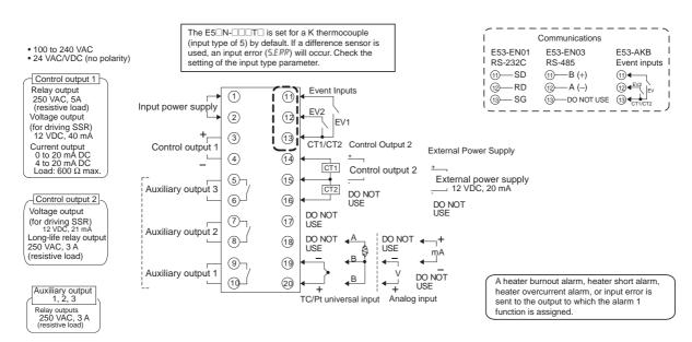
Since the voltage output (control output) is not electrically insulated from the internal wiring, one or other of the control output terminals must be left unearthed when using an earthed thermocouple thermometer. (Connection makes measurements unreliable due to sneak currents.)
