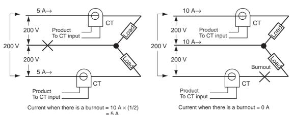
The heater burnout current when there is a burnout at the common is as follows:
