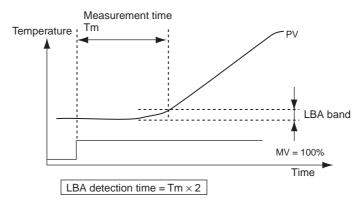
3. Set the LBA Detection Time parameter to two times the measured time.
