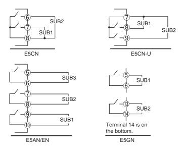
ALM1, 2, 3 can be output to auxiliary output 1, 2, 3, or changed with the advanced function setting level.
