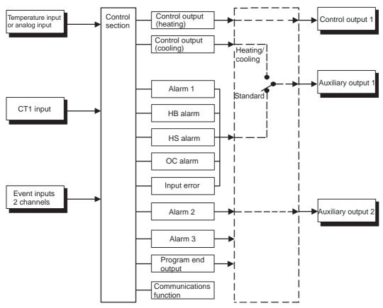
**Note** Functions can be assigned individually for each output by changing the set values for the Control Output 1 Assignment, the Auxiliary Output 1 Assignment, and the Auxiliary Output 2 Assignment parameters in the advanced function setting level.
