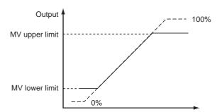
**Note** When the manual MV limit is enabled, the manual MV will be restricted by the MV limit.
