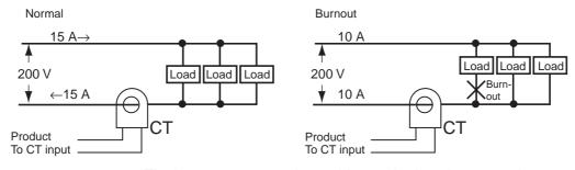
The heater power supply provides 15 A when the current is normal, and 10 A when there is a burnout, so the heater burnout detection current is calculated as follows:
