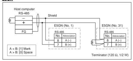
• The RS-485 connection can be either one-to-one or one-to-N. A maximum of 32 Units (including the host computer) can be connected in one-to-N systems. The maximum total cable length is 500 m. Use a shielded, AWG24 to AWG14 (cross-sectional area of 0.205 to 2.081 mm²) twisted-pair cable for the E5CN, E5EN, or E5AN. Use a shielded, AWG24 to AWG18 (cross-sectional area of 0.205 to 0.823 mm²) twisted-pair cable for the E5GN.
