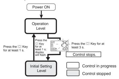
To move from the operation level to the initial setting level, press the  $\square$  Key for at least three seconds with any parameter displayed except for the Auto/Manual Switch parameter.
