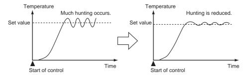
When the temperature (PV) falls short of the set point for the PID constants when using AT or ST in normal mode, executing AT or ST in RT mode tends to improve performance.
