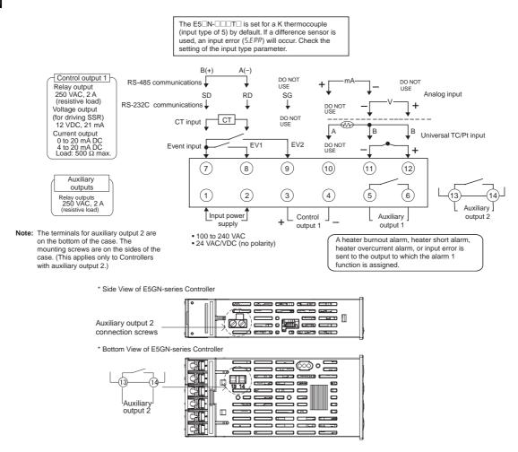
Since the voltage output (control output) is not electrically insulated from the internal wiring, one or other of the control output terminals must be left unearthed when using an earthed thermocouple thermometer. (Connection makes measurements unreliable due to sneak currents.)
