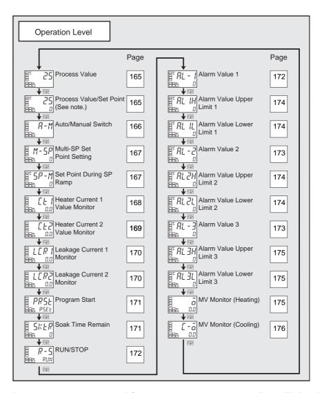
**Note** For details on the displays of Controllers with a No. 3 display (E5AN/EN), refer to *Process Value/Set Point* on page 165.
