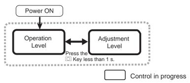
To move to the adjustment level from the operation level, press the  $\ \ \ \$  Key once.
