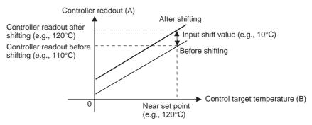
Figure 2 Illustration of 1-Point Shift
