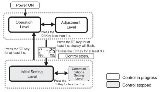
This level is displayed immediately after the power is turned ON.
