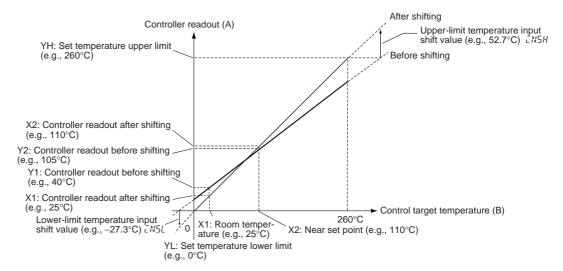
Figure 3 Illustration of 2-Point Shift
