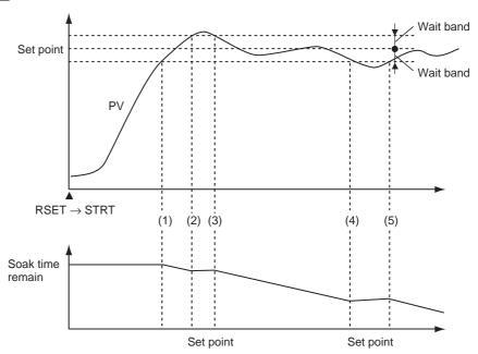
The wait band is the band within which the process value is stable in respect to the set point. The soak time is measured within the wait band. The timer that measures the soak time operates only when the process value is within the wait band around the set point (i.e.,  $SP \pm wait band$ ). In the following diagram, the timer will be stopped between the start and (1), (2) and (3), and (4) and (5) and will measure the time only between (1) and (2), (3) and (4), and (5) and the end.
