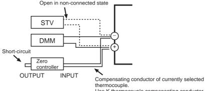
Use K thermocouple compensating conductor for E, R, S, B, W, and PLII thermocouples and for an infrared temperature sensor.
