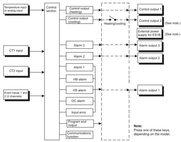
Note Functions can be assigned individually to each output by changing the set values for the Control Output 1 Assignment, Control Output 2 Assignment, Auxiliary Output 1 Assignment, Auxiliary Output 2 Assignment, and Auxiliary Output 3 Assignment parameters in the advanced function setting level.
