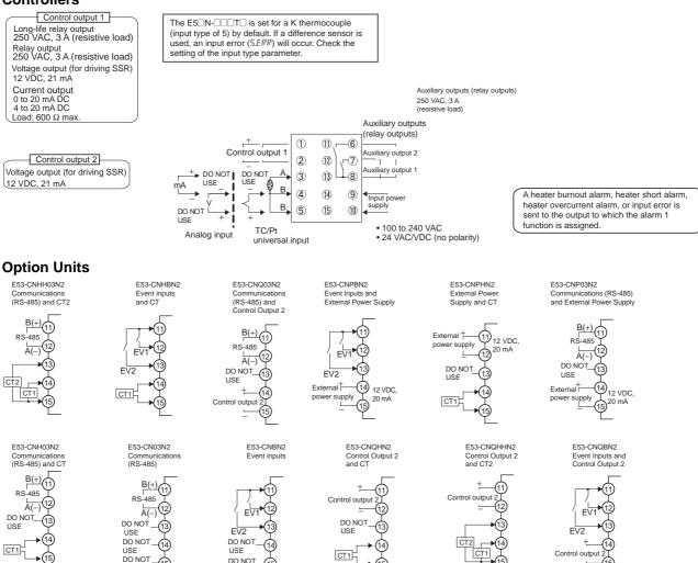
Since the voltage output (control output) is not electrically insulated from the internal wiring, one or other of the control output terminals must be left unearthed when using an earthed thermocouple thermometer. (Connection makes measurements unreliable due to sneak currents.)
