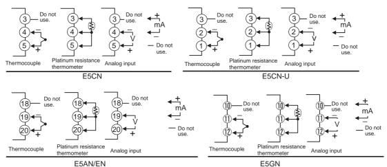
When extending the thermocouple lead wires, be sure to use compensating wires that match the thermocouple type. When extending the lead wires of a platinum resistance thermometer, be sure to use wires that have low resistance and keep the resistance of the three lead wires the same.
