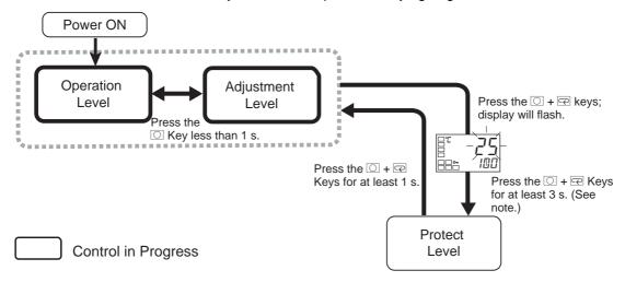
To move from the operation level to the protect level, press  $\bigcirc$  and  $\bigcirc$  Keys for three seconds (see note) or more.
