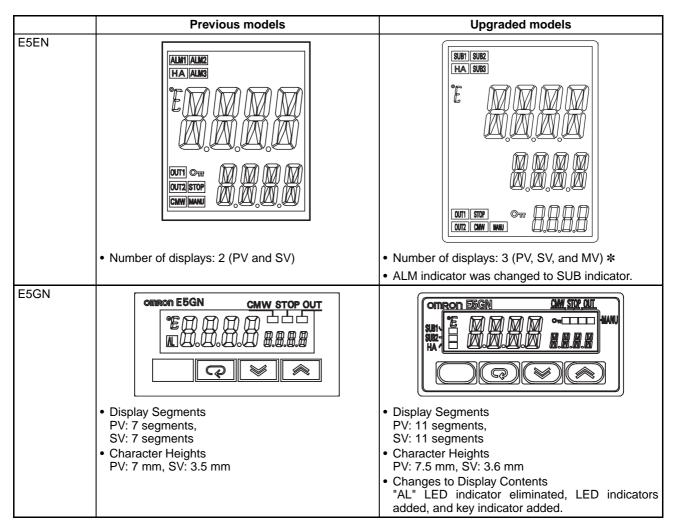
\* A 2-level display is set when shipped from the factory. A 3-level display is activated if parameters are initialized.
