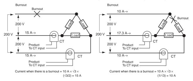
The heater burnout current when there is a burnout at the load line is as follows:
