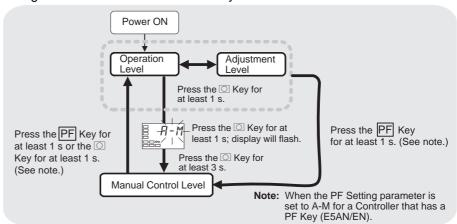
To move from the operation level to the manual control level, press the  $\bigcirc$  Key for at least three seconds with the Auto/Manual Switch parameter displayed. In addition, this operation can be performed using the PF Key by setting the PF Key parameter (advanced function setting level) to A-M (Auto/Manual). For details on the setting method, refer to *4-13 Performing Manual Control*.
