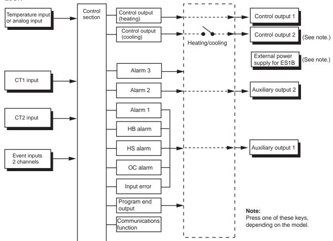
**Note** Functions can be assigned individually for each output by changing the set values for the Control Output 1 Assignment, the Control Output 2 Assignment, the Auxiliary Output 1 Assignment, and the Auxiliary Output 2 Assignment parameters in the advanced function setting level.
