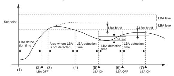
If the control deviation is reduced in the area between 1 and 2 (i.e., the set point is approached) and the amount the control deviation is reduced is at least equal to the LBA band, the loop burnout alarm will remain OFF.
