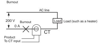
The heater power supply provides 5 A when the current is normal, and 0 A when there is a burnout, so the heater burnout detection current is calculated as follows:
