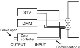
Compensating conductor of currently selected thermocouple.
