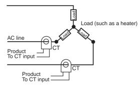
V connecting lines: Refer to the following diagram for CT installation positions.
