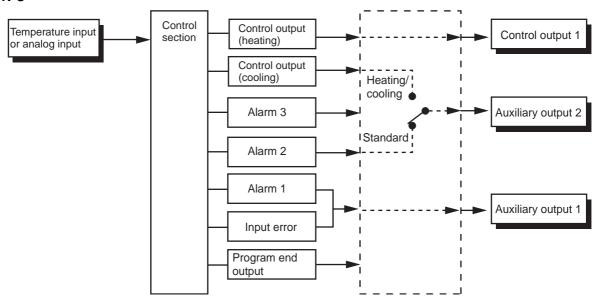
**Note** Functions can be assigned individually for each output by changing the set values for the Control Output 1 Assignment, the Auxiliary Output 1 Assignment, and the Auxiliary Output 2 Assignment parameters in the advanced function setting level.
