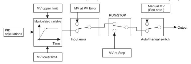
**Note** When the Manual MV Limit Enable parameter is set to ON, the setting range will be the MV lower limit to the MV upper limit.
