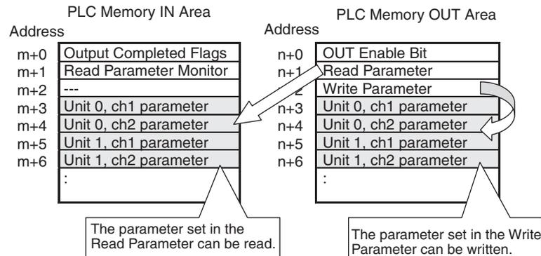
Note a) The parameters that can be specified are the ones that can be changed during operation.
