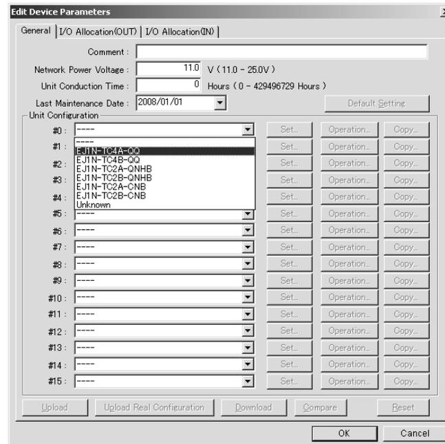
**Note** Click the Set Button to display the Edit Unit Parameters Window and then edit the parameters of the corresponding Temperature Controller (refer to page 93). Click the Operation Button to display the Operation Commands for Units Window, and control the corresponding Temperature Controller (refer to page 91). Click the Copy Button to copy parameters between Temperature Controllers simply by specifying the copy source and destination. (refer to page 89).
