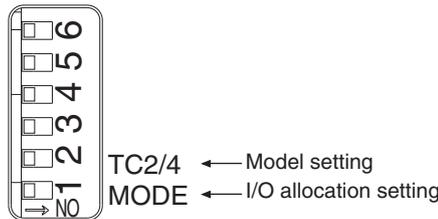
The Temperature Controller connection configuration and I/O allocations can be set using simple I/O allocations or I/O allocations from the Configurator.
