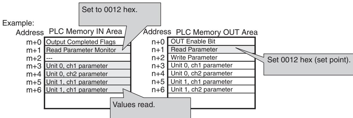
**Programming Example for Reading Parameters**
