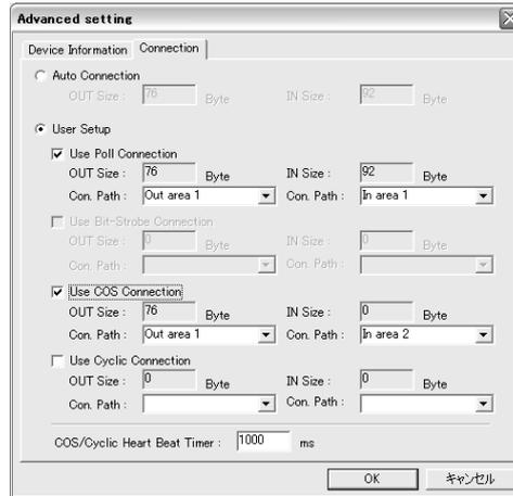
**Note** The output for the Poll connection and the output for the COS or Cyclic connection are sent in the same frame. Therefore, the same output size must be set for both connections when using a Poll and COS combination, or a Poll and Cyclic combination. When a COS or Cyclic connection are used, always set a dummy output size, and set the same connection path that is used for the Poll connection.
