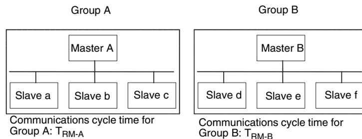
In Networks with two masters, the communications cycle time for the entire Network will be the sum of the communications cycle times for both groups.
