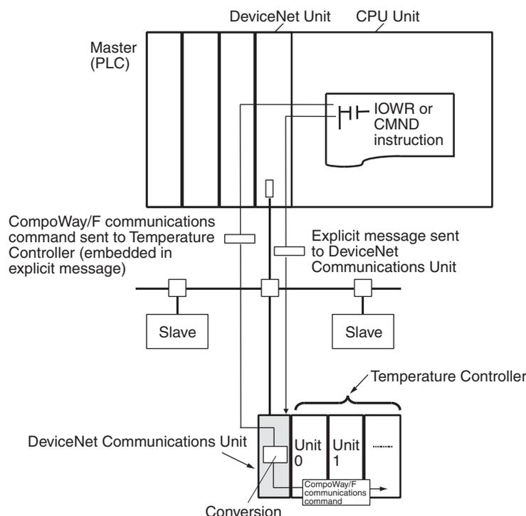
**Note** This manual describes the contents of explicit messages that can be sent to DeviceNet Communications Units. For details on the methods of sending explicit messages, refer to the operation manual for the DeviceNet Unit being used as the master.
