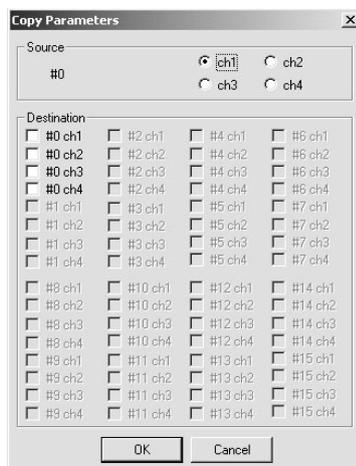
3. Select the channel from which to copy, specify the unit number and channel as the copy destination, and then click the **OK** Button. The parameters will be copied and the display will return to the Edit Device Parameters Window for the DeviceNet Communications Unit.
