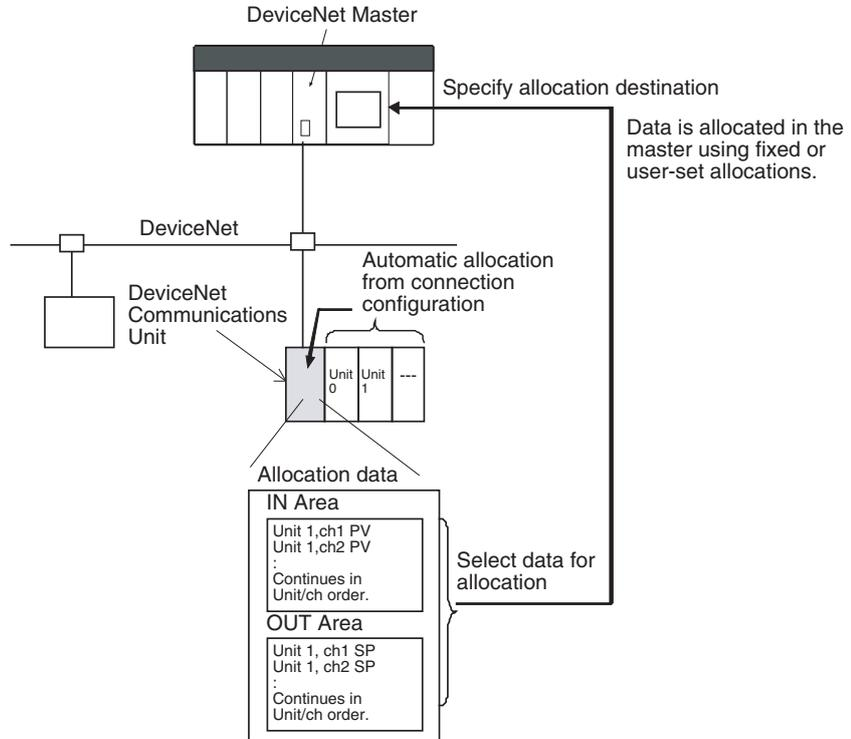
**Note:** The above allocation data is automatically allocated according to the connection configuration.
