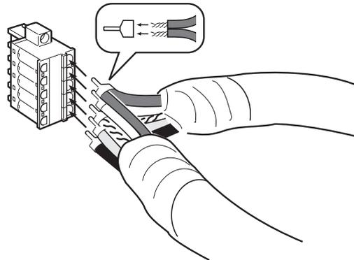
Crimp the two lines together that are to be inserted into the same hole using a special crimp terminal, as shown in the following diagram.
