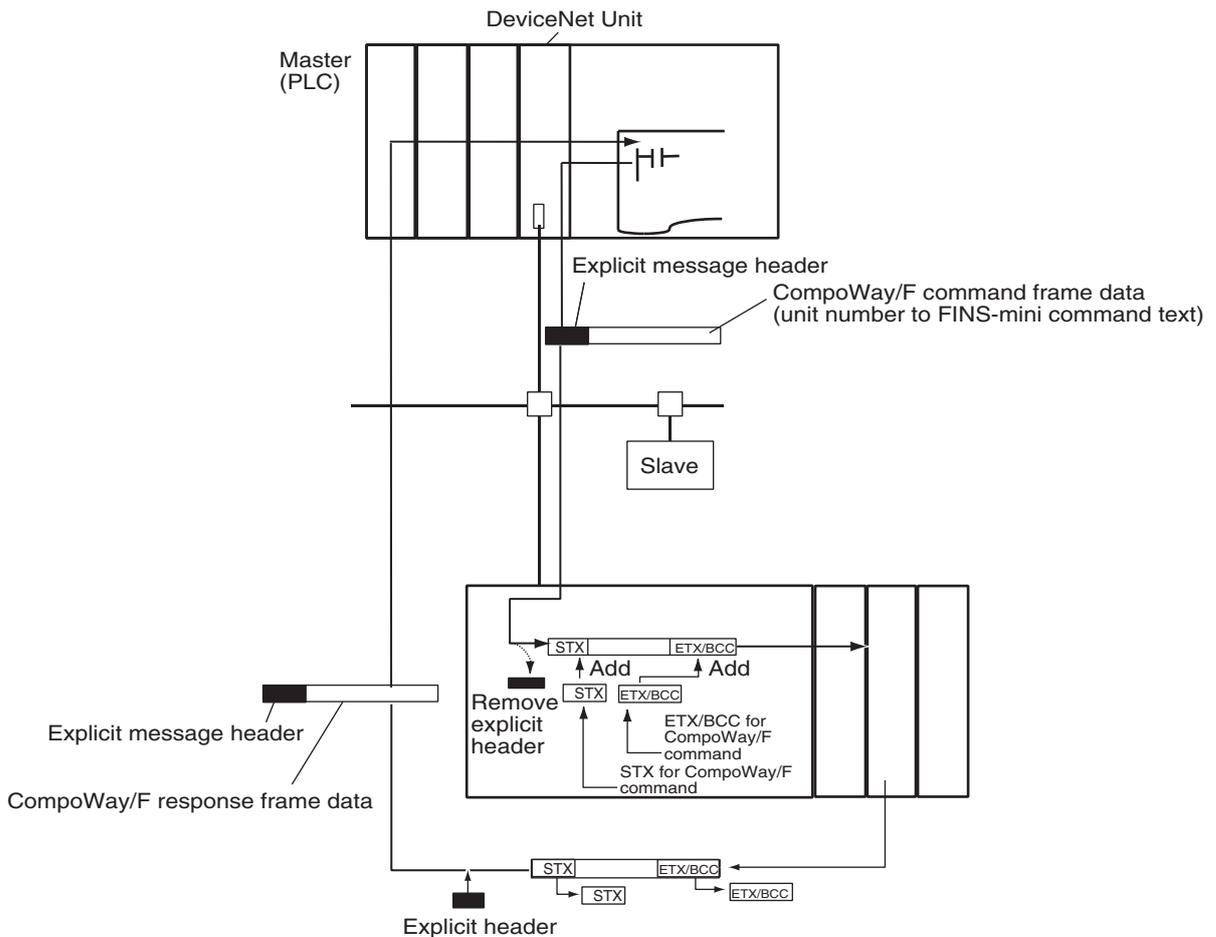
**Note** The CompoWay/F frames can be expressed in binary (hexadecimal) (CompoWay/F binary commands) or ASCII (CompoWay/F ASCII commands). Generally, CompoWay/F binary commands are used to minimize the number of operations. Always use CompoWay/F ASCII commands, however, when broadcasting or executing using a Read Controller Attribute (05 03).
