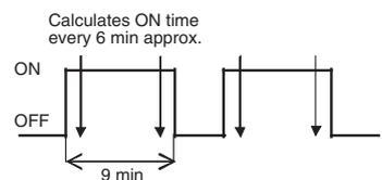
In the above diagram, the actual conduction time is 9 minutes  $\times$  2 = 18 minutes, but the status is ON four times when the measurement is taken, so the conduction time is calculated as 24 minutes.
