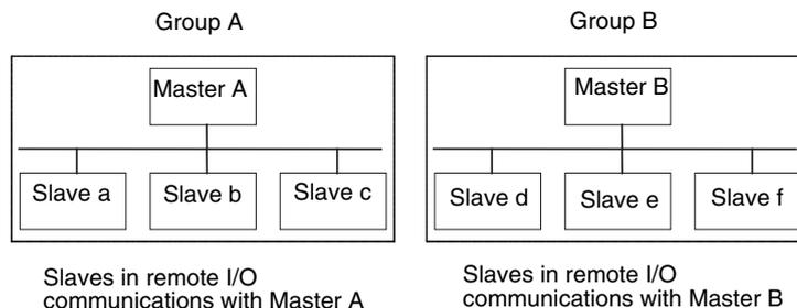
**Note** Although in the above diagram the slaves are separated into two separate groups for each master for convenience, the actual physical positions of the slaves in the Network are irrelevant.
