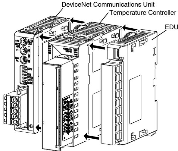
Connect the End Unit to the right end and connect the DeviceNet Communications Unit to the left end.
