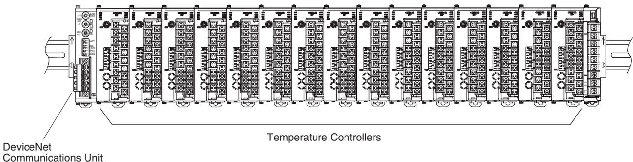
The DeviceNet Communications Unit differentiates each of the connected Temperature Controllers according to communications unit numbers (0 to F: 0 to 15 decimal). The Temperature Controllers can be connected in any order. The communications unit number of each Temperature Controller is set using the rotary switch on the front panel of the Temperature Controller. Always set a unique communications unit number for each Temperature Controller.
