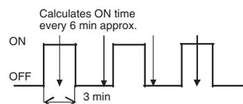
In the above diagram, the actual conduction time is 3 minutes  $\times$  3 = 9 minutes, but the status is ON only twice at the time the measurement is taken, so the conduction time is calculated as 12 minutes.
