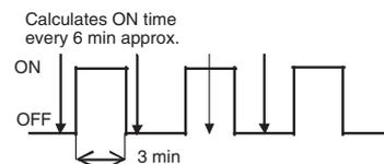
In the above diagram, the actual conduction time is 3 minutes  $\times$  3 = 9 minutes, but the status is ON only once at the time the measurement is taken, so the conduction time is calculated as 6 minutes.
