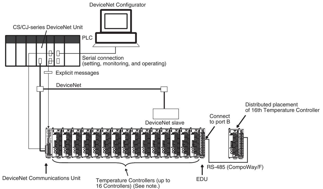
Note: Up to 16 Temperature Controllers can be connected to one DeviceNet Communications Unit. Use distributed placement via RS-485 for the 16th Temperature Controller.
