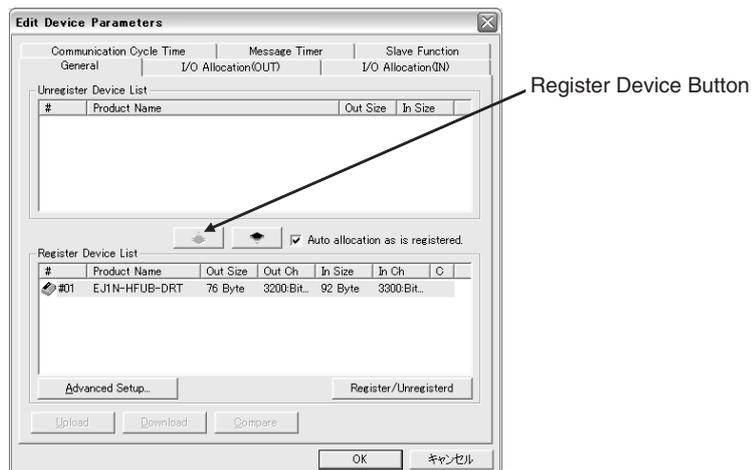
3. Select the **I/O Allocation (OUT)** and **I/O Allocation (IN)** Tab, and check that the allocation data created in the Edit Device Parameters Window for the DeviceNet Communications Unit parameters is registered in the master's allocated area (memory block 1 or 2).
