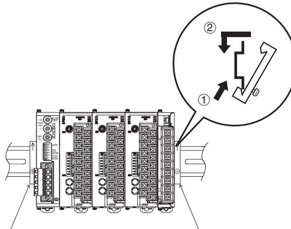
**Note** Always use two End Plates to clamp the Units together from both ends.
