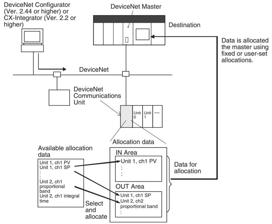
**Note:** Create the above allocation data using the Configurator's Edit Device Parameters and then download to the DeviceNet Communications Unit.
