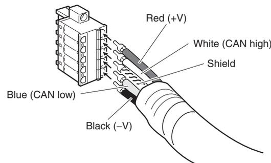
Colored stickers that match the colors of the lines to be inserted are provided on the Master Unit and slaves. Use these stickers to check that the lines are wired correctly. The colors correspond to the signal lines as follows:
