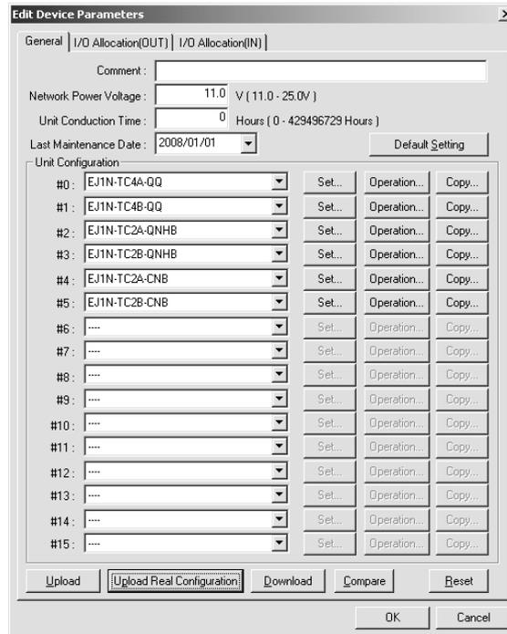
2. A window for editing the unit parameters of the corresponding Temperature Controller will be displayed.
