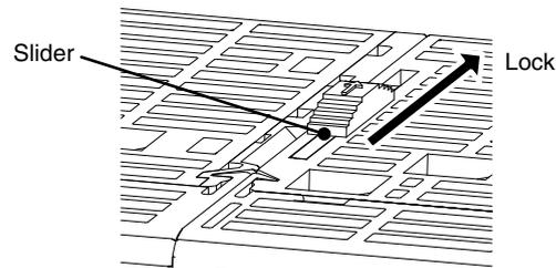
3. Attach the cover seal to the connector on the Unit on the left end of the EJ1.
