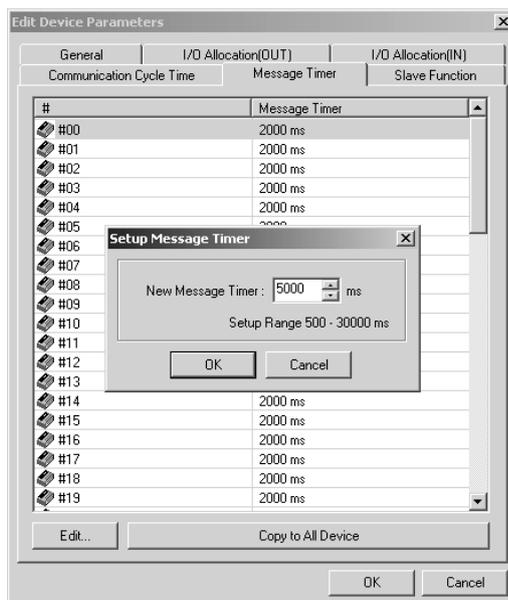
4. Click the **General** Tab in the Edit Device Parameters Window, and then click the **Download** Button. The parameters will be downloaded and the value for the message monitor timer of the DeviceNet Communications Unit will be changed.
