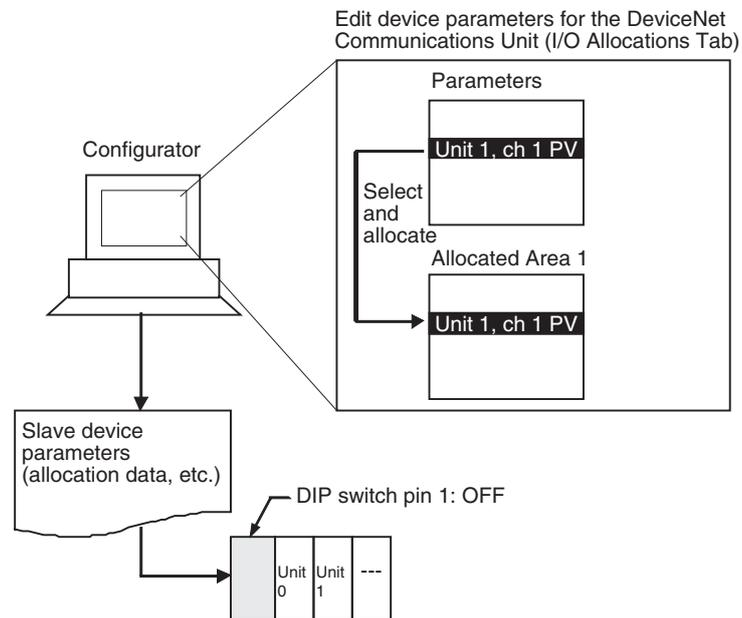
**Note** The maximum allocation size for the IN and OUT Areas (100 words) applies to the DeviceNet Communications Unit, and does not apply to the size of allocations in the Master Unit. For details on allocation sizes in the Master Unit, refer to the operation manual for the Master Unit being used.
