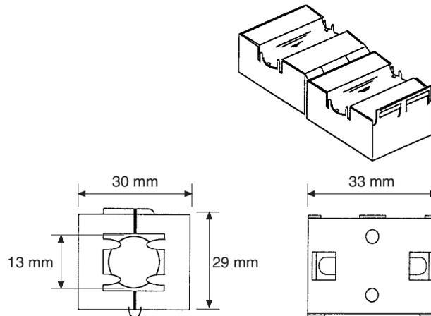
Ferrite Core (Data Line Filter): 0443-164151 (manufactured by Fair-Rite Products Co., Ltd.)
