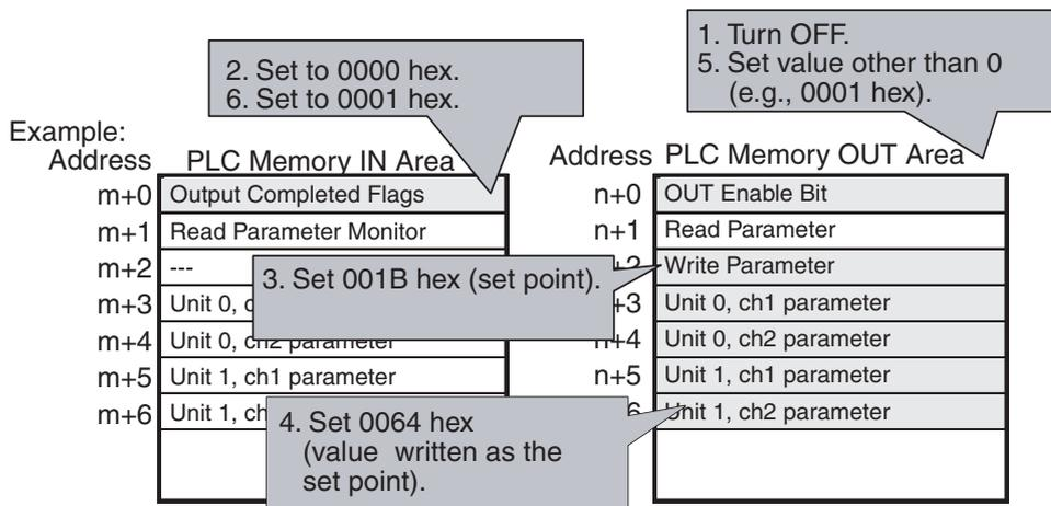
**Note** Always change the OUT Enable Bit to 0 before attempting to write parameters using expansion remote I/O. If writing is attempted while the bit is not 0, writing may be performed while the allocation number or write values are being set, and unintended values may be written.
