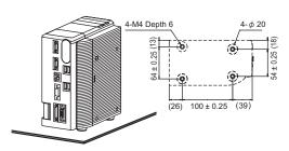
\* When mounting the controller on its bottom, it must be fixed without removing the feet to reserve ventilation path.
