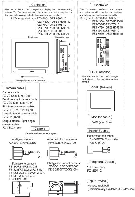
\* FZ-SC5M, FZ-S5M, FZ-SC5M2 and FZ-S5M2 can only be connected to FZ3-7\_\_-10 and FZ3-H7\_\_-10/FZ3-9\_\_-10/FZ3-H9\_\_-10.
