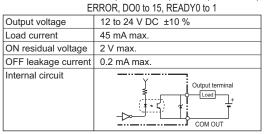
[Output] signals: When STGOUT0-3 are used, connect the COM IN terminal.
