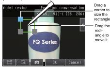
Check the area, press the [OK] Button, and then press the [TEACH] Button. The characteristic part and reference position for position compensation will be registered.
