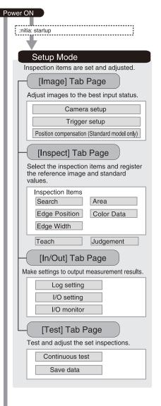
When a Sensor that is a:ready set up is connected
