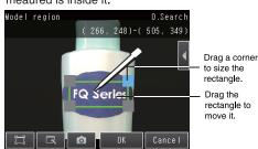
Check the area, press the [OK] Button, and then press the [TEACH] Button. Register the image as the measurement reference.
