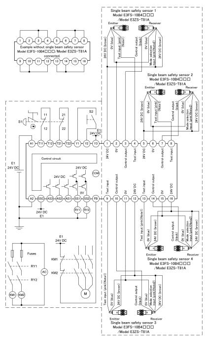
\$1 : Emergency-stop switch (positive opening contacts) (Model A165E, Model A22E)  $\bigodot$  : Reset switch KM1、KM2 : Magnetic contactor
