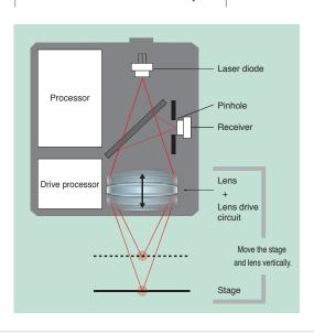
In a normal confocal model, a stage and lens are driven vertically to change the focal point. This requires a more complex structure, and the large number of parts interferes with downsizing. The use of a laser beam increases the chances of interference, and the received light waveform can be disrupted by the surface conditions within the small spot on the measurement object.
