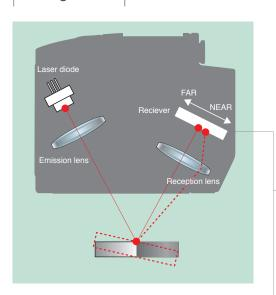
Triangulation measures the height of an object based on the position of the spot on a receiver (CCD or CMOS). The peak, center of gravity, and other features are calculated from the received light waveform to reduce error, but in principle, the received waveform is offset or disrupted due to differences in materials or inclination. This results in measurement error.
