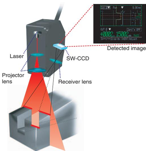
**Principle of line beam method**
