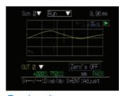
Trend monitor Time-series change of measurement data can be checked.
