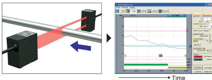
The trend of the measurement data and sudden change can be checked in the time-dependent graph, so that the appropriate action can be taken before defective goods are produced.
