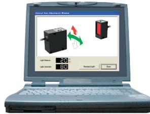
The direction of the sensor head's adjustment is graphically displayed. The adjustment conditions can be confirmed through the shapes of the light reception waveforms.
