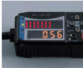
The Imaging Device light reception balance is displayed in the upper display and the amount of light received can be confirmed with numerical values underneath.
