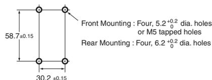
\* If the conduit size and ground terminal specifications are "with TS 1/2-14NPT ground terminal", the back mounting hole is 4-6.2 dia. <sup>+0.2</sup>/<sub>0</sub>.
