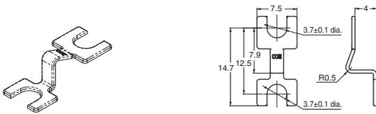
When attaching the Terminal Plate to the built-in switch terminal, the SPST-NO+NC contact can be converted to an SPDT contact.
