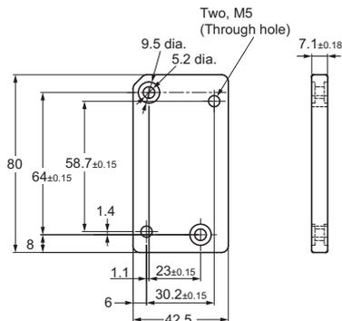
The Side mounting plate allows the actuator to be installed in the same position as the side mounting of the WL□-2N series.
