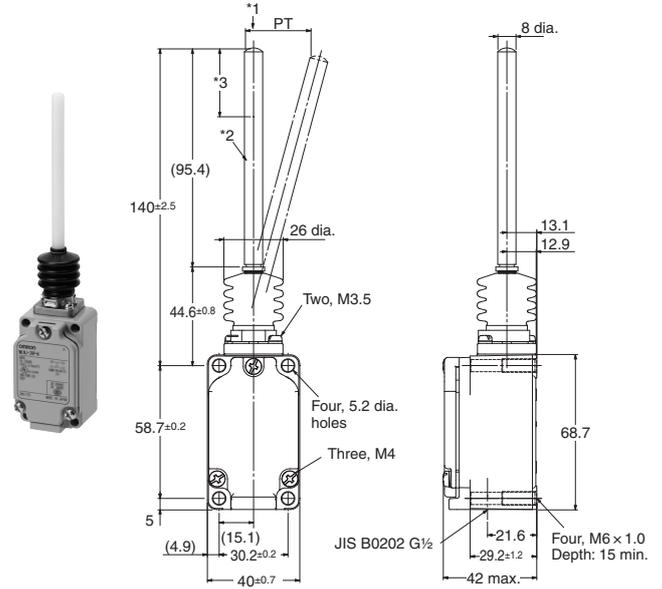
\*1. Do not operate the Switch in the direction of the axial center.
