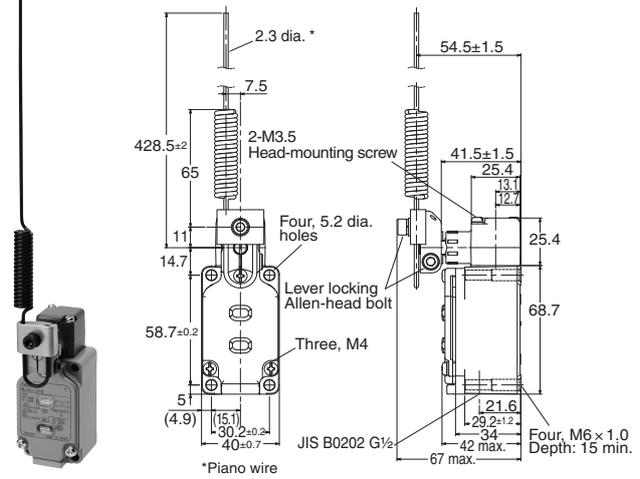
**Note:** Unless otherwise indicated, a tolerance of  $\pm 0.4$  mm applies to all dimensions.
