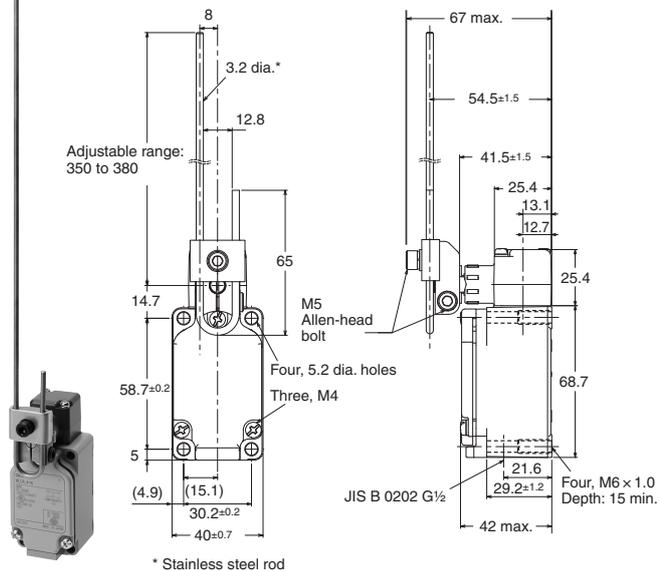
Adjustable Roller Lever (350 to 380 mm)
