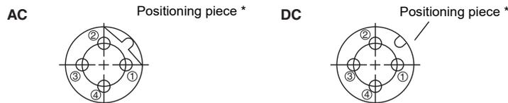
\* The position of the positioning piece is not always the same. If using an L-shaped connector causes problems in mounting, use a straight connector.
