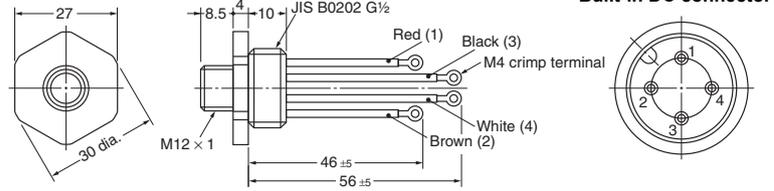
Note: 1. Each dimension has a tolerance of  $\pm 0.4$  mm unless otherwise specified.
