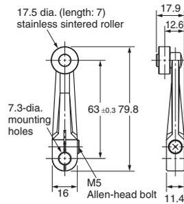
Note: Unless otherwise indicated, a tolerance of  $\pm 0.4$  mm applies to all dimensions.
