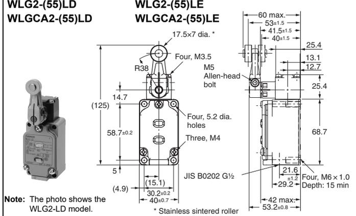
**Note:** Unless otherwise indicated, a tolerance of  $\pm 0.4$  mm applies to all dimensions.
