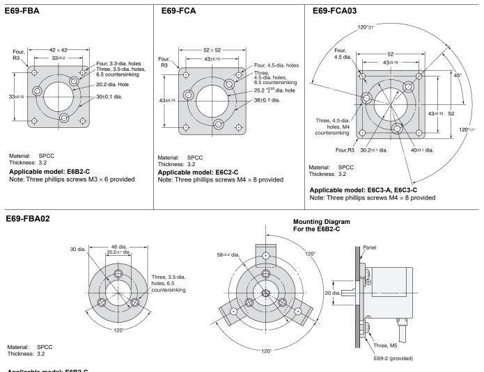
Applicable model: E6B2-C Note: Three phillips screws M3  $\times$  10 provided, E69-2 Servo Mounting Bracket provided
