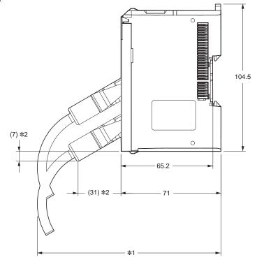
**\*1.** Depends on the connector to use. For MPS588-C: Approximately For MPS588-C: Approximately 120 mm For XS6G-T421-1: Approximately 130 mm **\*2.** Dimension for XS6G-T421-1. For MPS588-C, the connector does not protrude from the bottom of the Unit.
