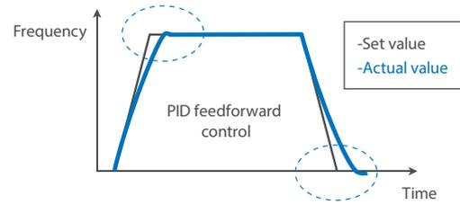
The NJ/NX/NY Controller executes sequence control, motion control, and I/O refreshing in the same control period. The calculation results of feedback control can be output in a short fixed cycle. This means the motor can constantly receive commands.
